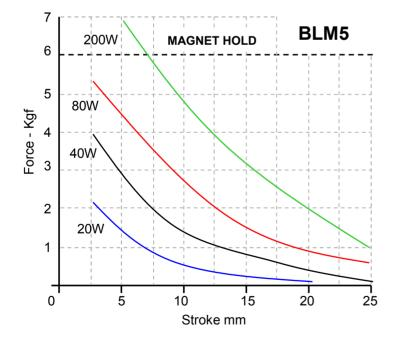
Forces shown are at working temperature Cold forces are higher
