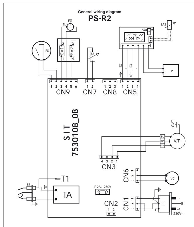
SA SAS SE VC VT I INTEGRATED ROOM PROBE SPLIT ROOM PROBE OUTSIDE PROBE (optional) COMBUSTION FAN TANGENTIAL FAN BATTERY HOLDER CONTROL BOARD PP SIT EA ER EV1 F IGNITION ELECTRODE
