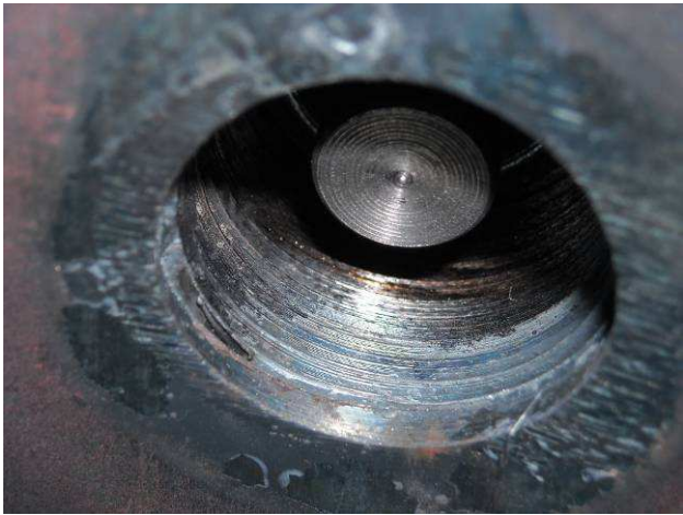
Fig. 12: Internal thread after IP66 test
