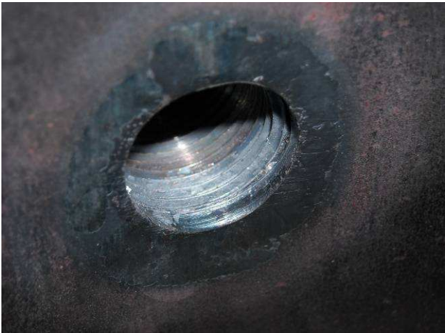
Fig.11: Internal thread after IP 66 test
