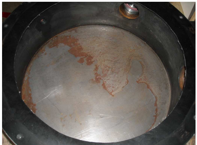
Fig. 10: Internal view after IP66 test
