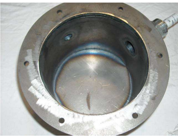
Fig. 10: Internal view after IP66 test
