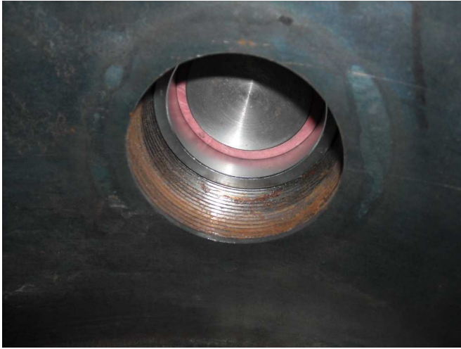
Fig.11: Internal thread after IP 66 test
