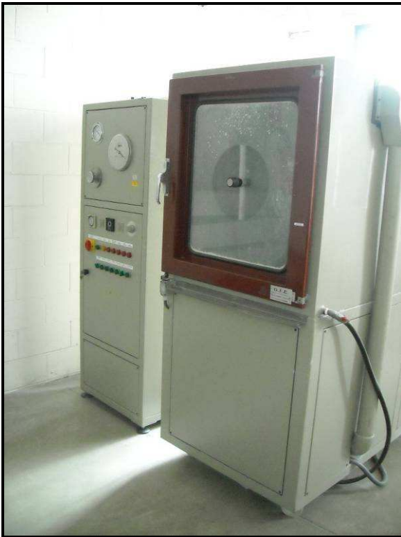
Typical setup for IP Dust penetration test
