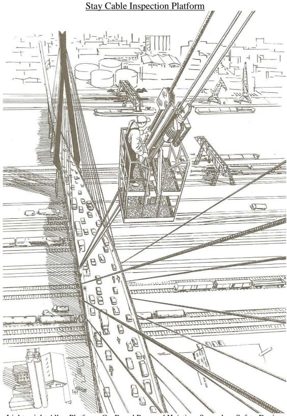
Lightweight Alloy Platform: On-Board Powered Hoisting: Secondary Safety Devise:
