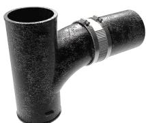
Butt ends of no hub cast iron pipe or fitting together inside the gasket until both are firmly seated against the center stop of gasket. Center the stainless steel shield assembly over the gasket.
