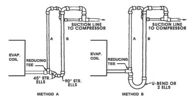
During the lower capacity running mode (compressor capacity control energised) oil will collect in the elbow or at the U-bend below pipe 'B'. This will divert the gas and oil so that it flows up pipe 'A' at a higher velocity.
