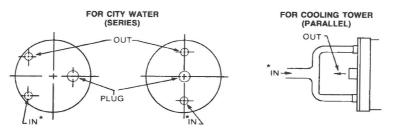
\* From compressor cooling coil (if equipped) and water regulating valve
