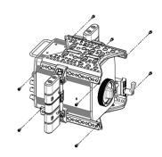
Start by attaching the plates to the camera. Make sure that the sides of the Mounting Plates (1) are aligned with each other.
