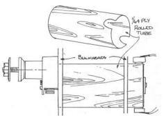
Make the tube the length of the motor and cut slots for the brush housings. The slots act as an anti-rotation device. Another trick is
