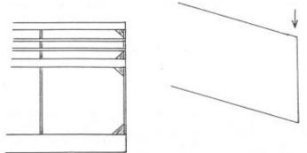
With the grain parallel to either side, it's not doing any good. As soon as there is any strain on it, the grain will split.
