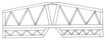
If you're worried about having the lumps showing through the covering, you can use a combination of these two. Put in the needed ribs and put in  $1/8" \ge 1/16"$  diagonals that don't touch the covering.
