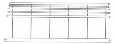
If you touch one wing tip on landing, the whole wing panel will try to parallelogram.
