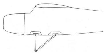
Like the trunnion block gear, this type also flexes out. Smaller diameter wire can be used than with the torsion bar landing gear of the wing. Use 1/8", 5/32", or 3/16" (for big planes), in wing torsion bar gear while 3/32" or 1/8" will work with this type of fuselage gear. There are all sorts of variations on this and different ways of doing it, but this is a pretty good landing gear.
