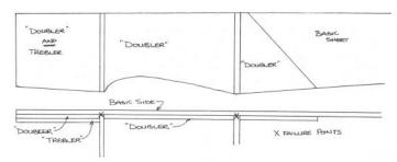
With the above construction, the plane comes in, bounces and breaks. There you have it - a fishead, lying on the flying field.
