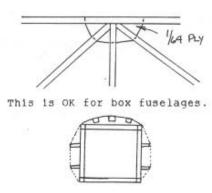
and you want to make it bulletproof, take 1/64" ply and gusset the inside of all joints. It adds hardly anything to the weight, but adds a tremendous amount of strength. The method to the side is okay for box
