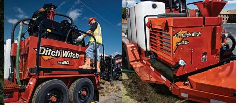
By reclaiming, recycling and reusing drilling mud, you retain profits that others are literally throwing away. You'll profit even more with the Ditch Witch® MR90, the most advanced, most productive mud recycler on the market. The MR90 can mix and recycle drilling mud as well as handle spoils, for exceptionally costeffective production. Among its many exclusively cost-efficient features: It has the fastest setup time on the market and it's the only mud recycler you can transport full of fluid.
