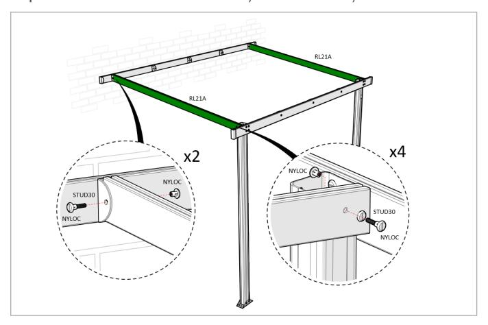
**Step 6** - Attach RL21 between front assembly and wall assembly
