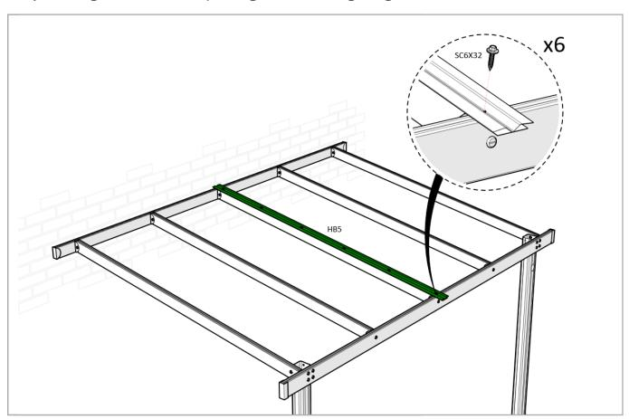
Step9 - Insert roof sheet into each side of HB5 and fix as shown
