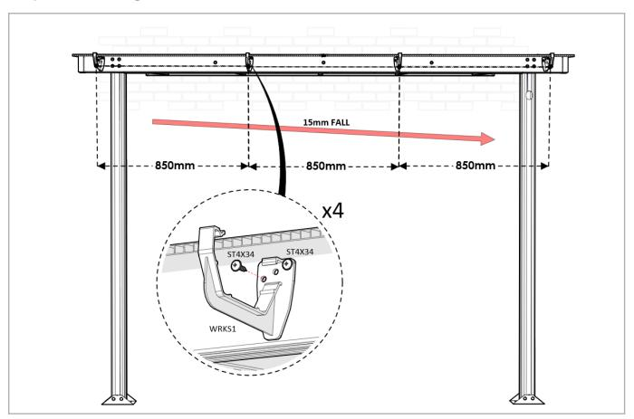
**Step 12** - Insert gutter, then connect waste-pipe and end caps
