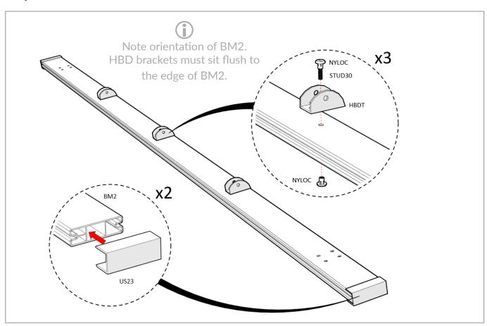
Step 3 - Fix RL22 assembly to wall
