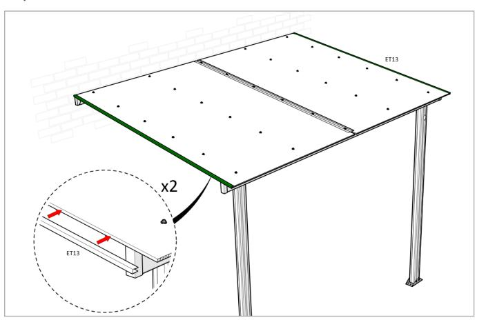
**Step 11** - Attach gutter brackets to front of BM2
