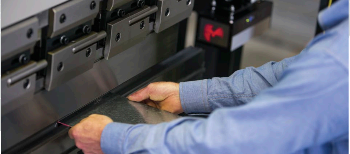
Close proximity protection enables safe handling of the work piece during high speed closing.
