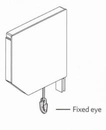
Locate the Crook Hook into the fixed eye and hold handle straight then rotate to wind up, or down as required.
