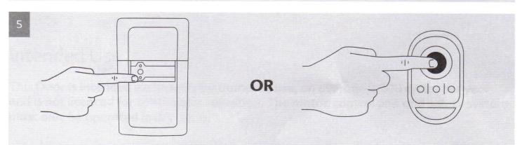
If the OSE safety system has a fault or fails to operate the door can be brought down by pressing and holding the down button on the control receiver board or by keeping the black button held down on the downward cycle of the operator key-fob.
