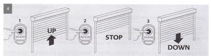
During the up or down cycle you can stop the door by simply pressing the black button on the key-fob. The next press of the black button on the key-fob will send the door in the opposite direction from which it was moving.
