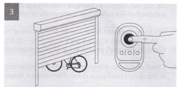
During the closing cycle if the door detects an obstruction it partially reverses and stops. The remote control receiver will emit a warning light flashing rapidly to confirm it has hit an obstacle. Remove the obstacle and press the black button again to close the door.
