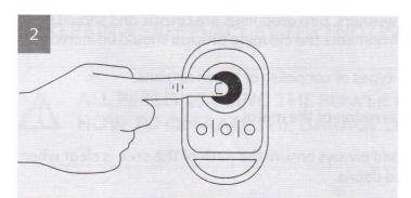
Press the large black button in the centre of the hand held transmitter (key-fob) for 1 second and the door will start to move to the fully open or closed position and stop. By pressing the black button again the door will perform the opposite sequence and stop.
