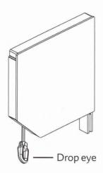
Locate the Crook Hook into the drop eye and hold handle at 45 degrees then rotate to wind up, or down as required.
