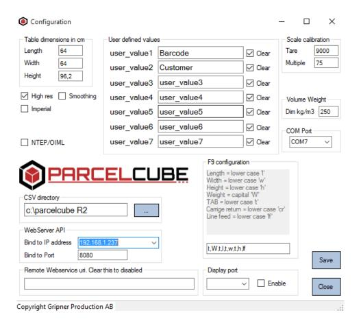
Chose the COM port in the drop down box named COM Port that corresponds with the Parcelcube serial port.
