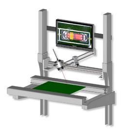
**Configuration B**: In-line HD Camera with 22" Full HD monitor, XY floating stand with 4-directions Tilt unit. **Application:** In-line Visual Inspection of assembled PCBs after Pick & Place and/or after AOI.
