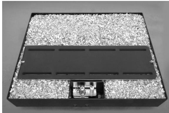
Typical burner showing black insulation pad in position and vermiculite fill, ready to lay ceramics. The pilot cut-out is normally in the centre at the front. As an alternative a side pilot cut-out is sometimes supplied.
