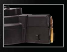
To function test the tension relief device, with a fully loaded magazine, the last cartridge should be able to depress  $\sim 1/8$ " with finger pressure. There may be a slight click noise when this occurs, it is normal. If the cartridge does not move inspect the tension relief device to ensure that debris is not obstructing it, and that the spring is in position.
