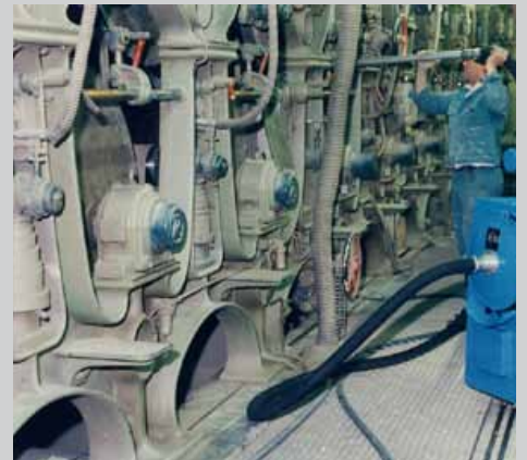
Factory cleaning, vacuum extraction of paper dust
