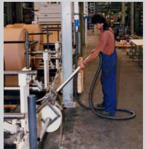
Cleaning of machines for decoration paper
