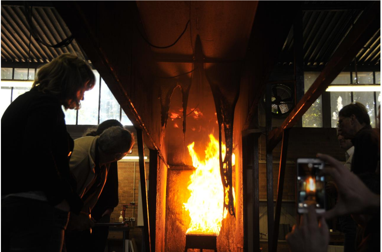
Figure 4.2.5.5: Material draping and dropping out up to 2 meter mark
