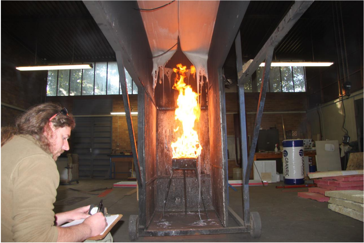
Figure 4.2.4.3: Molten material dropping out within Fire Source Area
