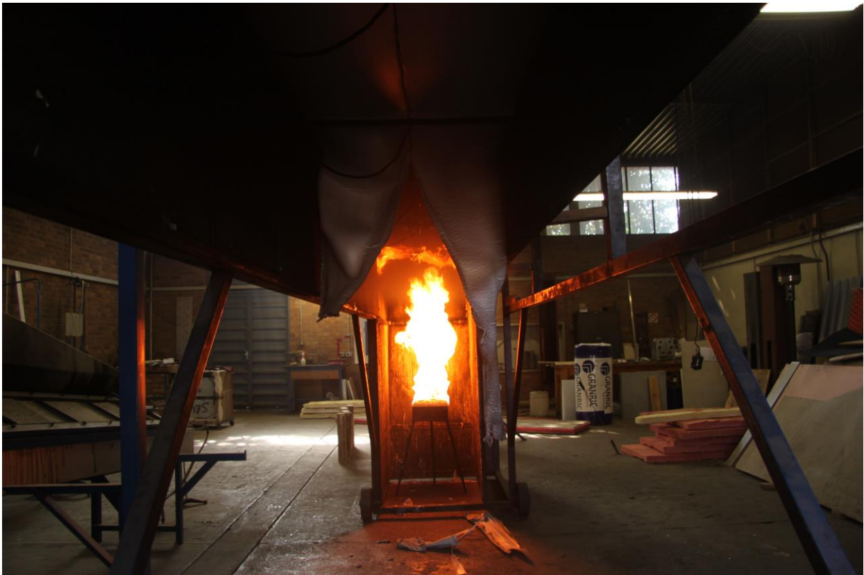
Figure 4.2.1.4: Material dropping out and draping up to 4 meters
