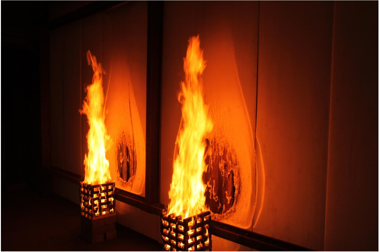
Figure 4.4.5: Molten material starting to flow down
