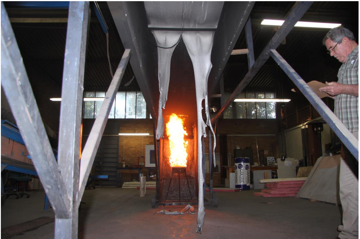
Figure 4.2.3.6: Material draping up to 4 meter mark
