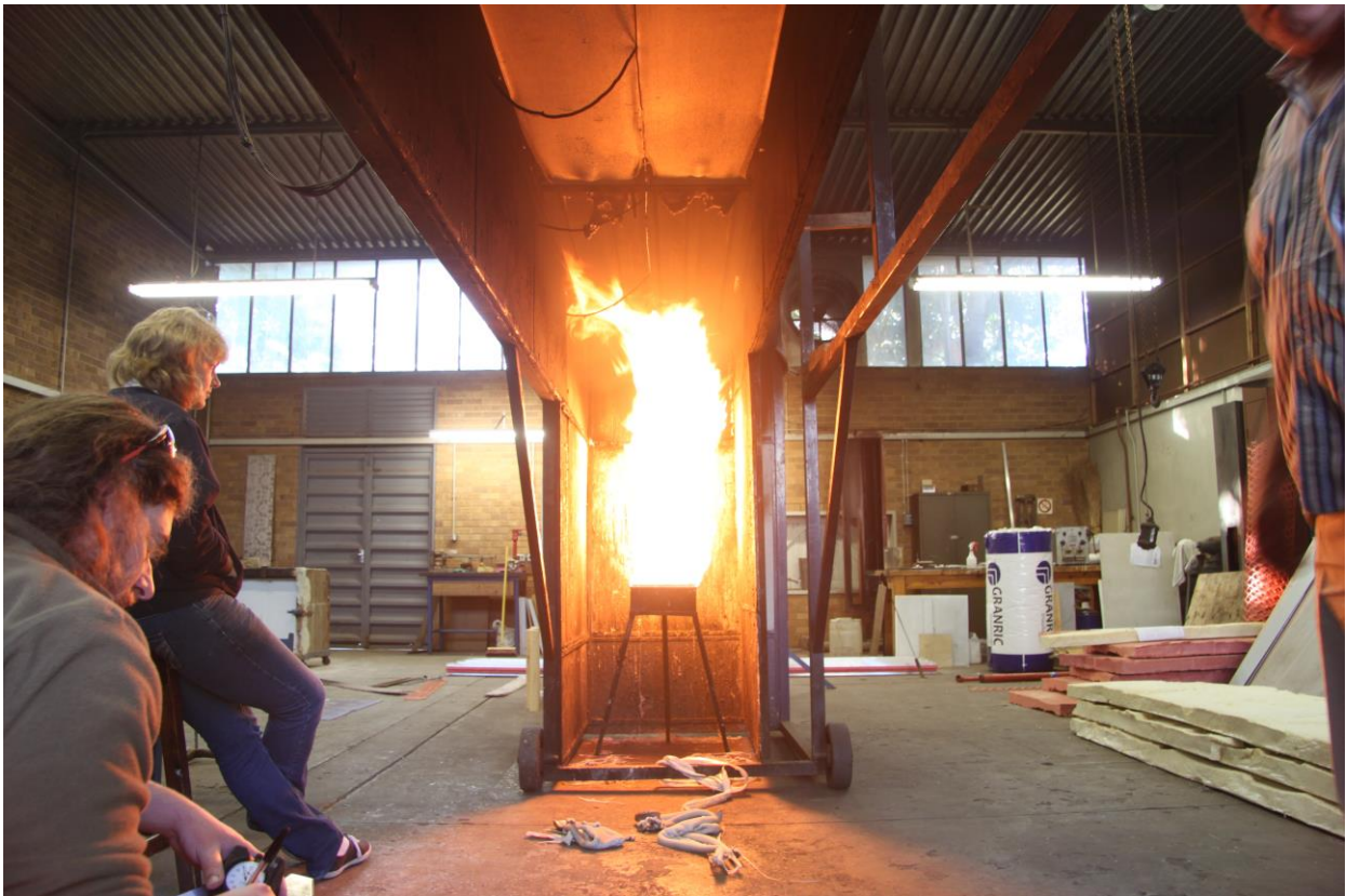
Figure 4.2.4.4: Softened material dropping out up to 2 meter mark
