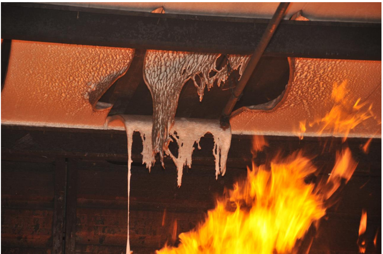
Figure 4.3.4: Molten material above Fire Source starts to flow
