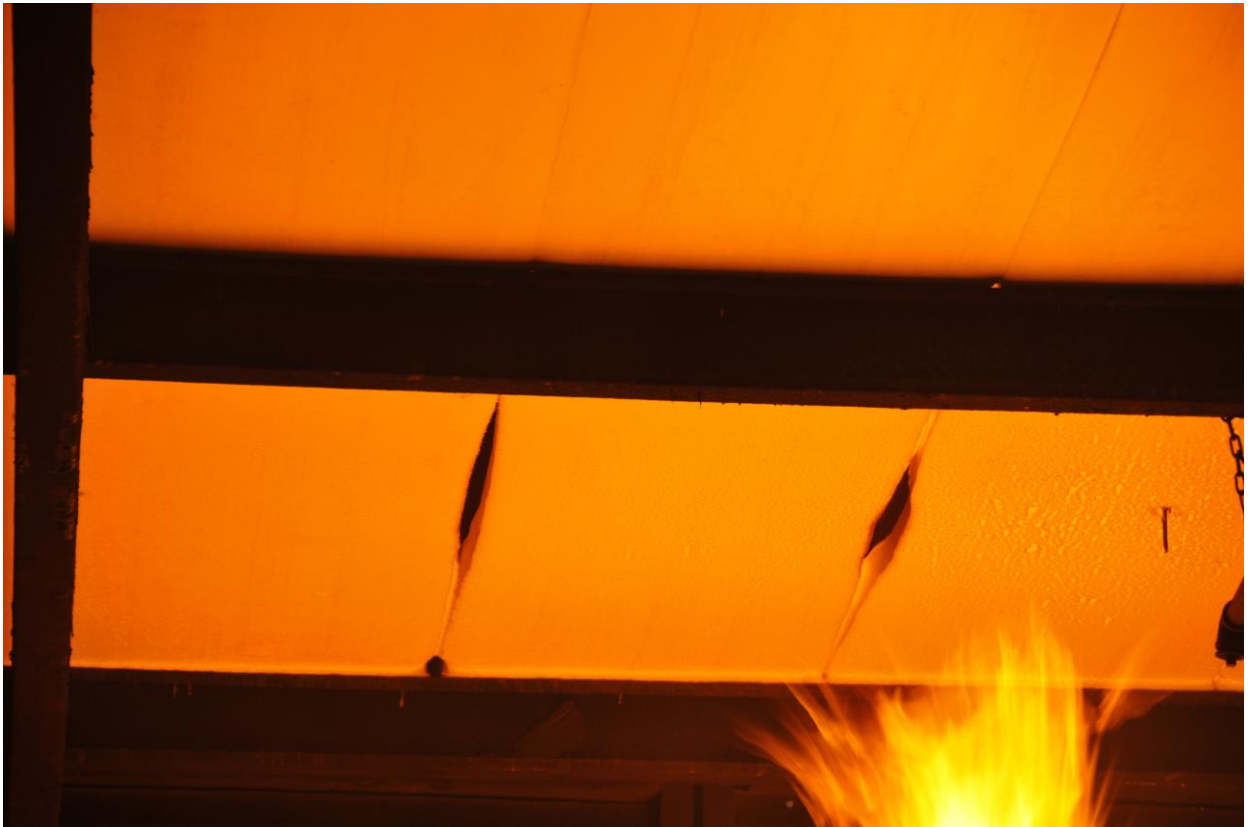
Figure 4.3.3: Surface coagulation visible and joints separating due to shrinkage
