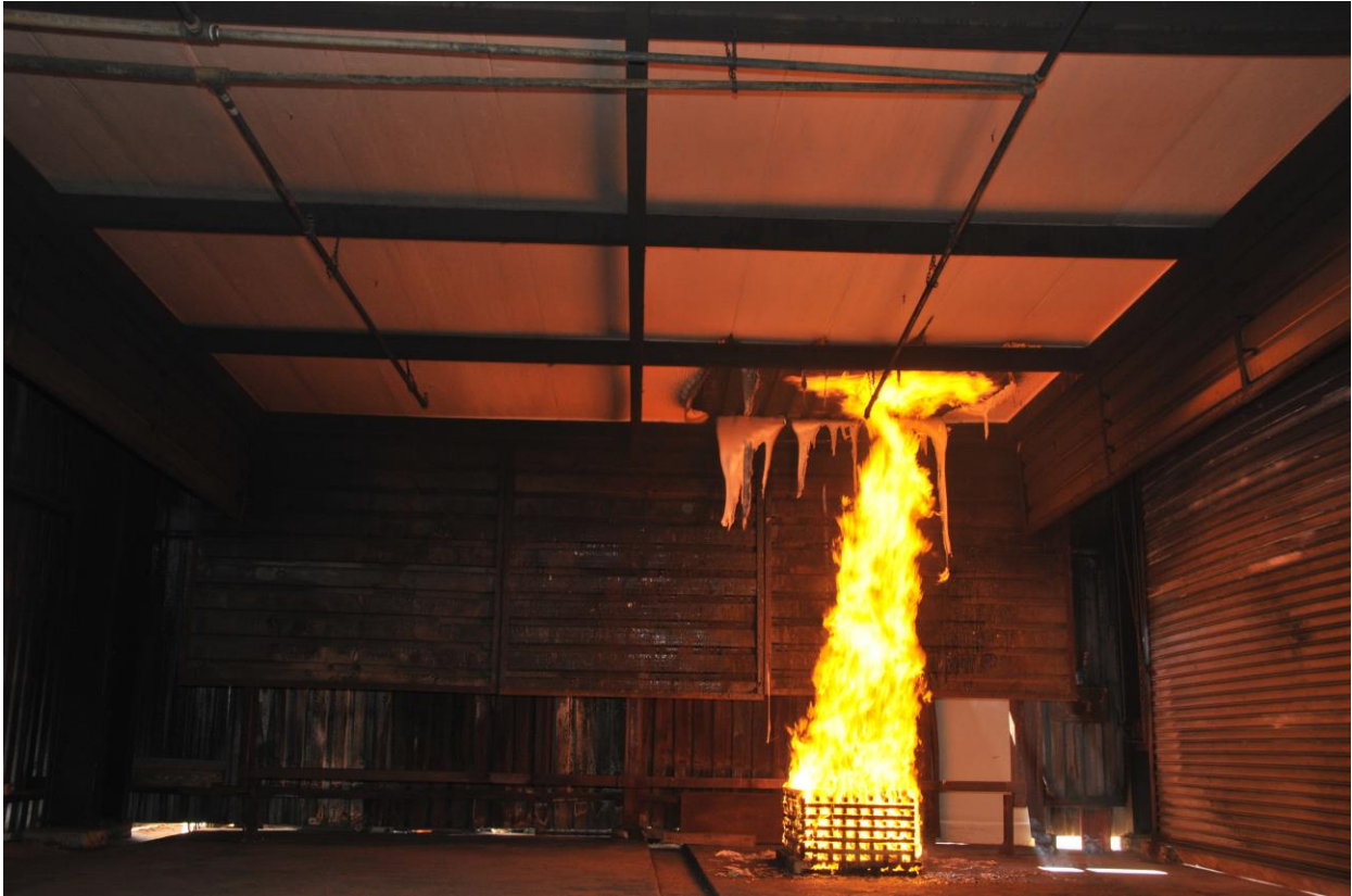
Figure 4.3.5: Material above Fire Source draping and dropping out
