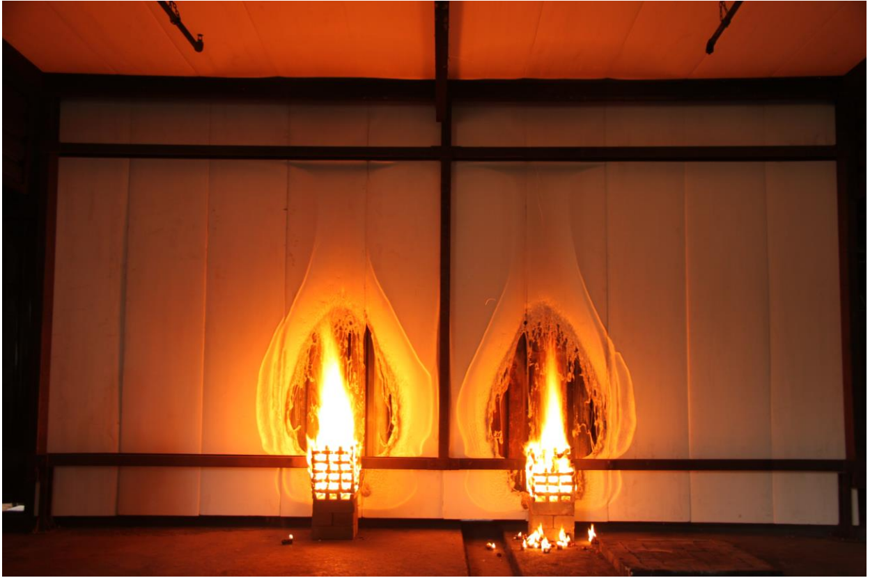
Figure 4.4.7: Cribs starting to collapse – No ignition occurred
