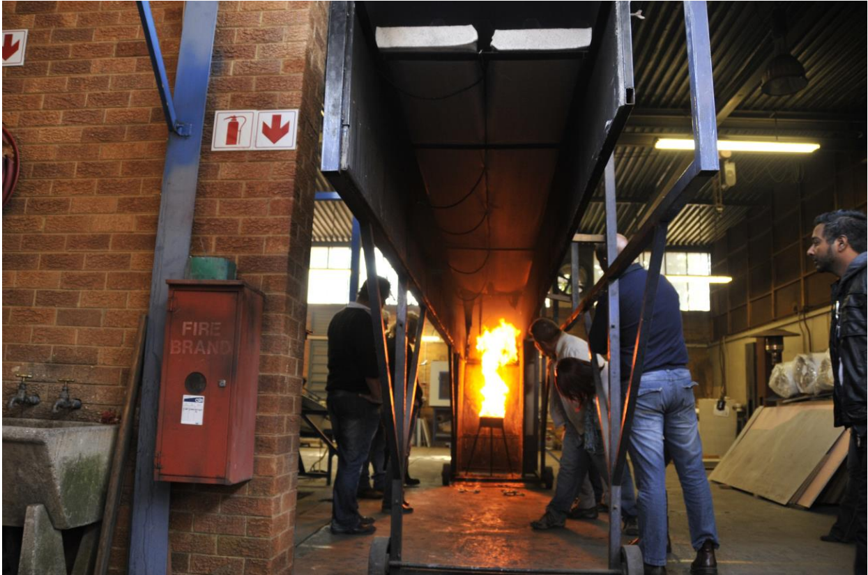
Figure 4.2.5.7: All material up to 2 meter mark dropped out
