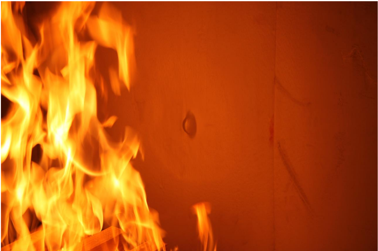
Figure 4.4.2: Material melting and bubble forming behind Crib
