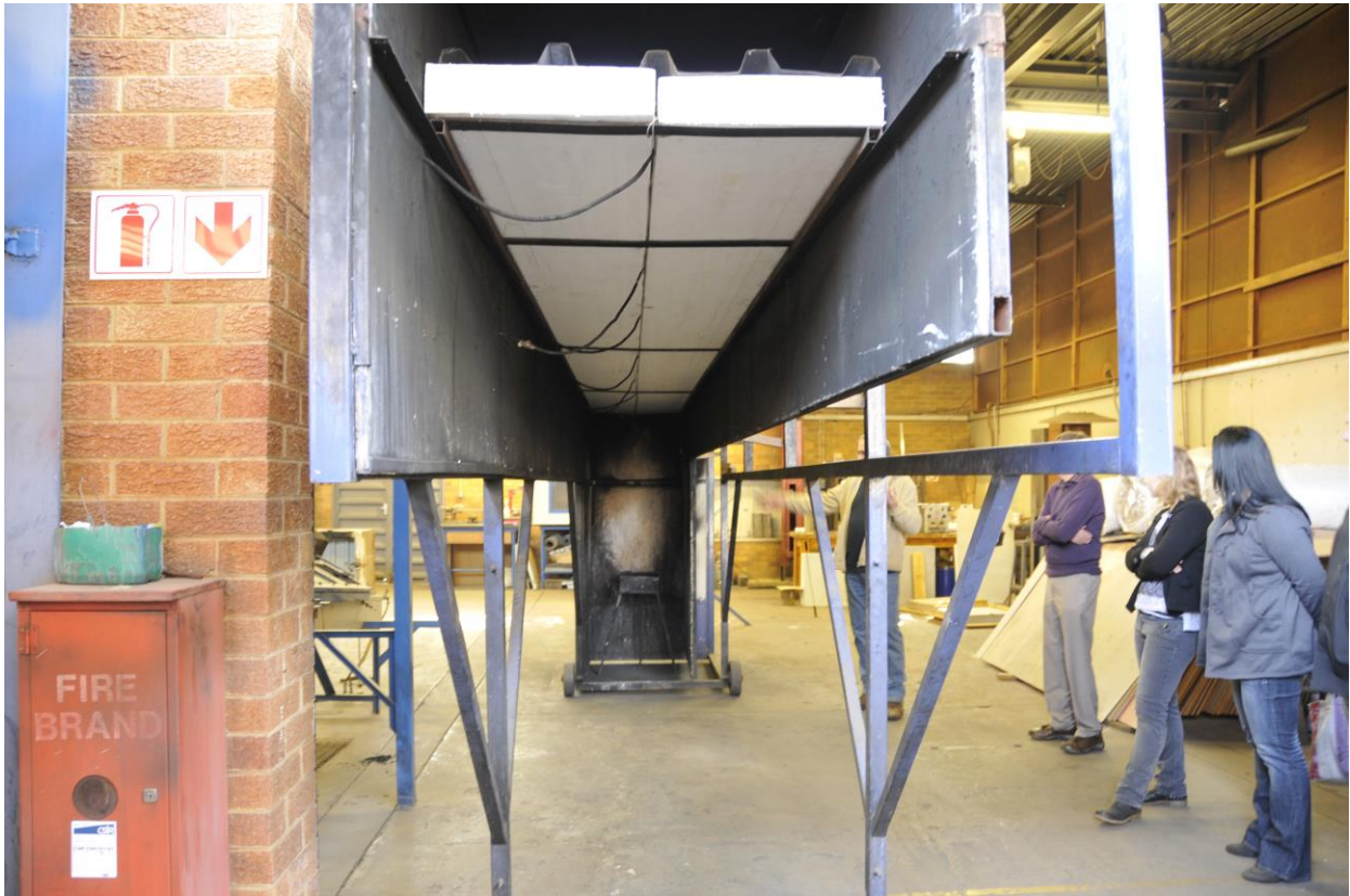
Figure 4.2.5.1: The test installation prior to ignition of the Fire Source
