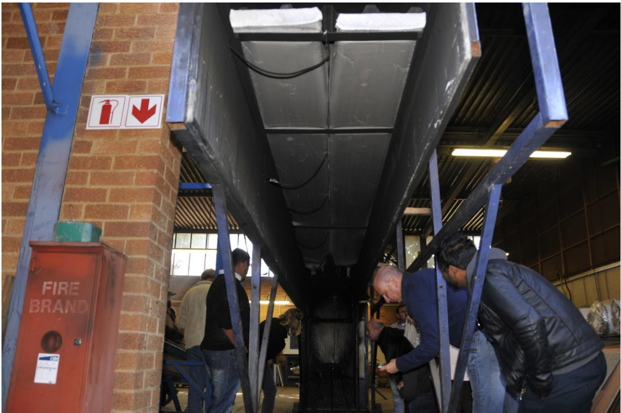
Figure 4.2.5.8: Test specimen at conclusion of SANS 10177 – 10 test
