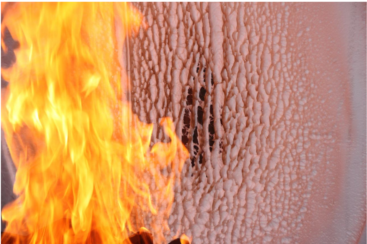
Figure 4.4.4: Coagulation of material exposing sheeting
