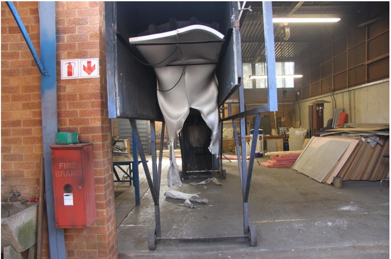
Figure 4.2.1.6: Test specimen at conclusion of SANS 10177 - 10 test
