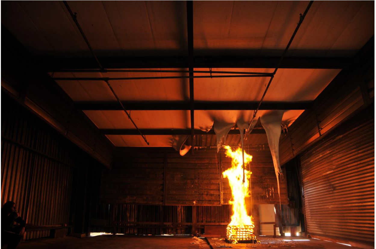
Figure 4.3.7: Fire Source (Crib) starting to collapse – Boards draping up to 3 meter mark
