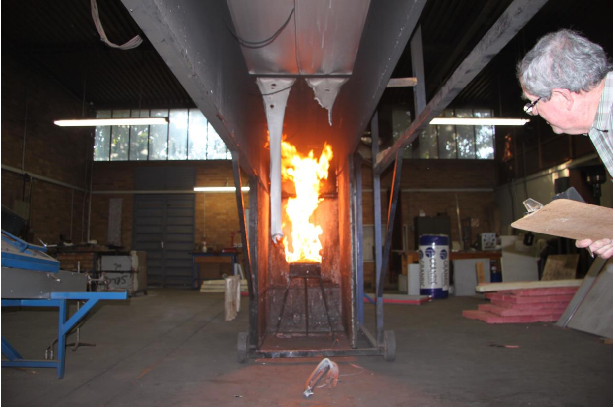
Figure 4.2.3.5: Material draping and dropping up to 2 meter mark
