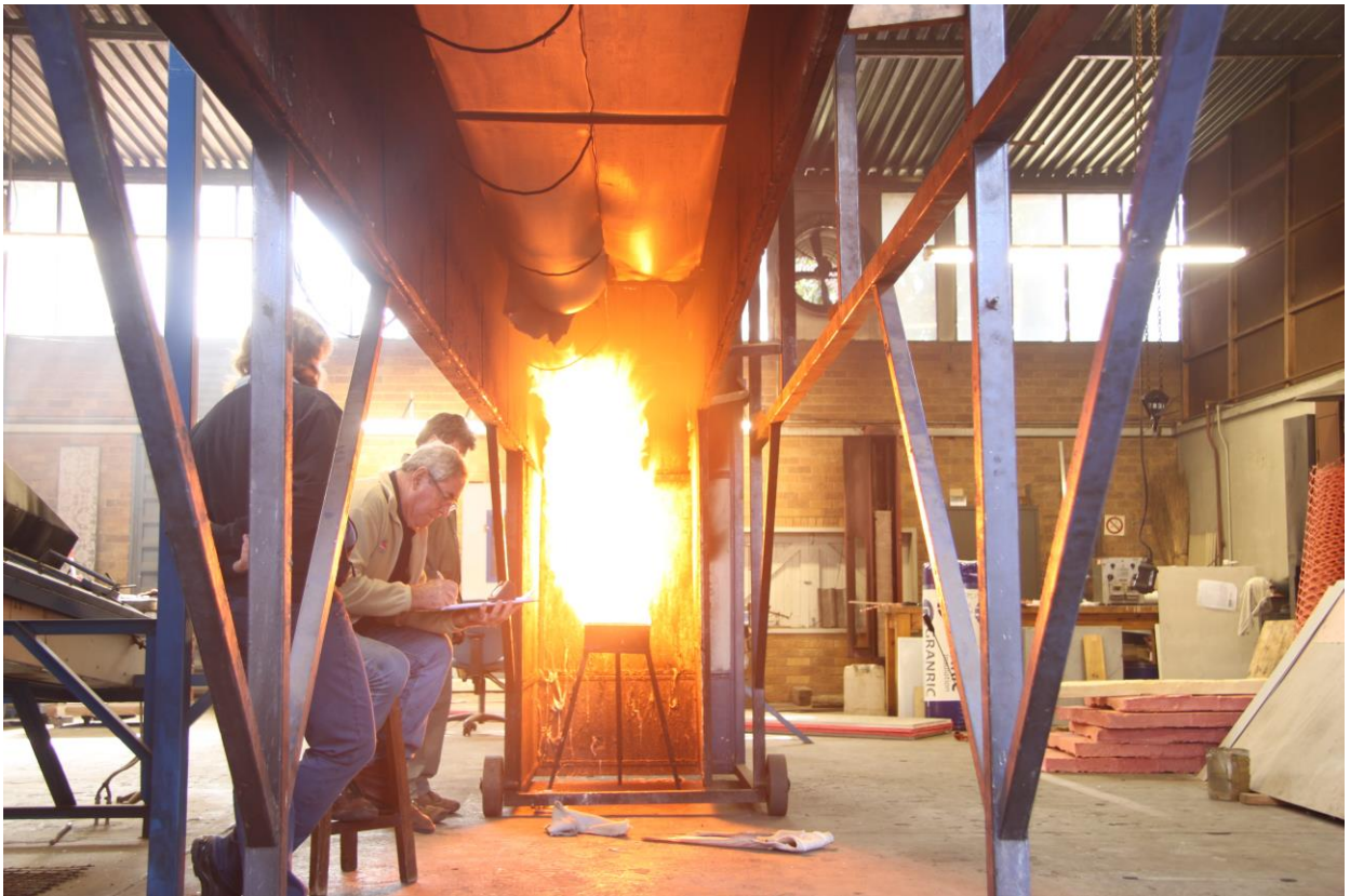
Figure 4.2.1.4: Heat damage and material draping up to 2 meters
