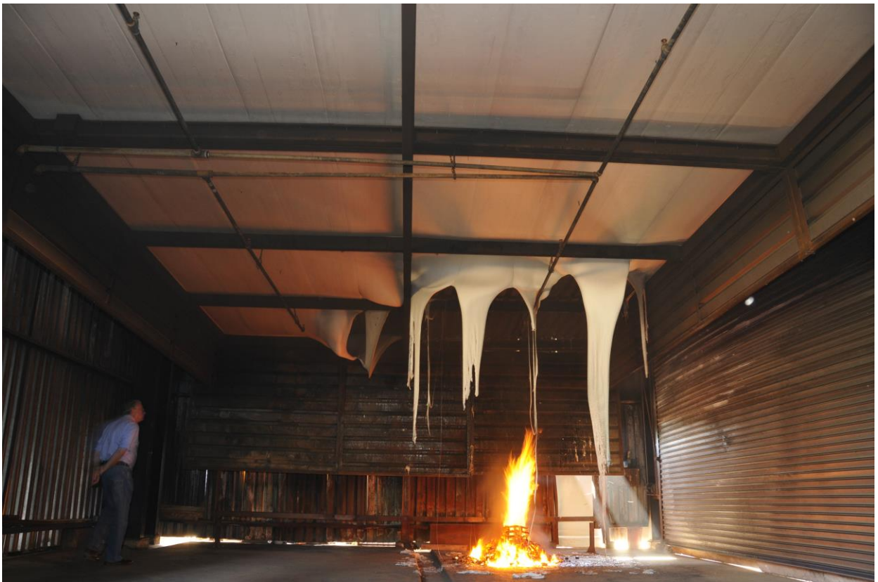
Figure 4.3.8: Fire Source (Crib) completely collapsed – Boards draping up to 4 meter mark
