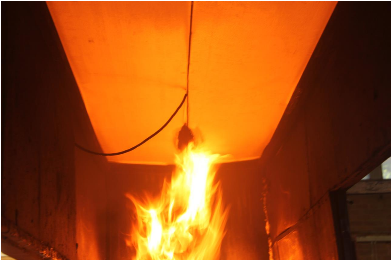
Figure 4.2.1.2: Heat damage above Fire Source with joint opening
