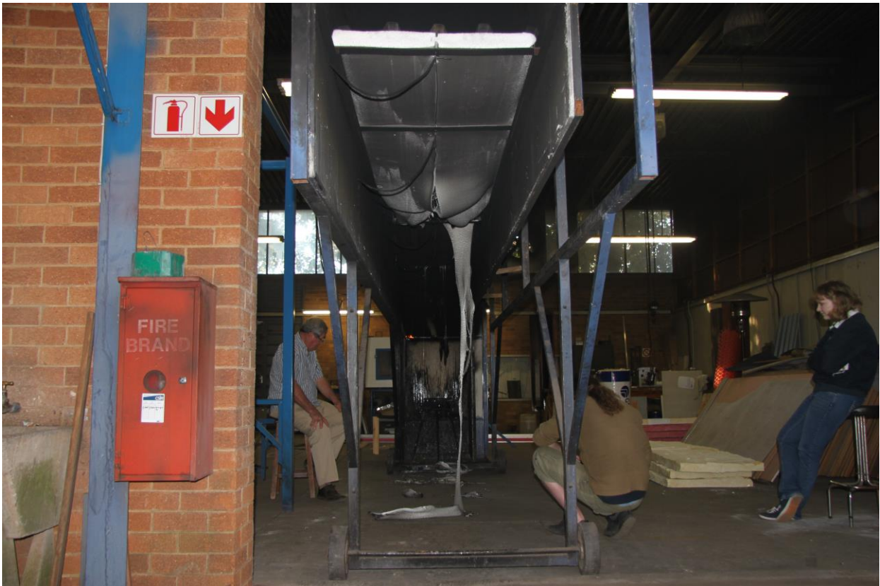
Figure 4.2.4.8: Test specimen at conclusion of SANS 10177 - 10 test
