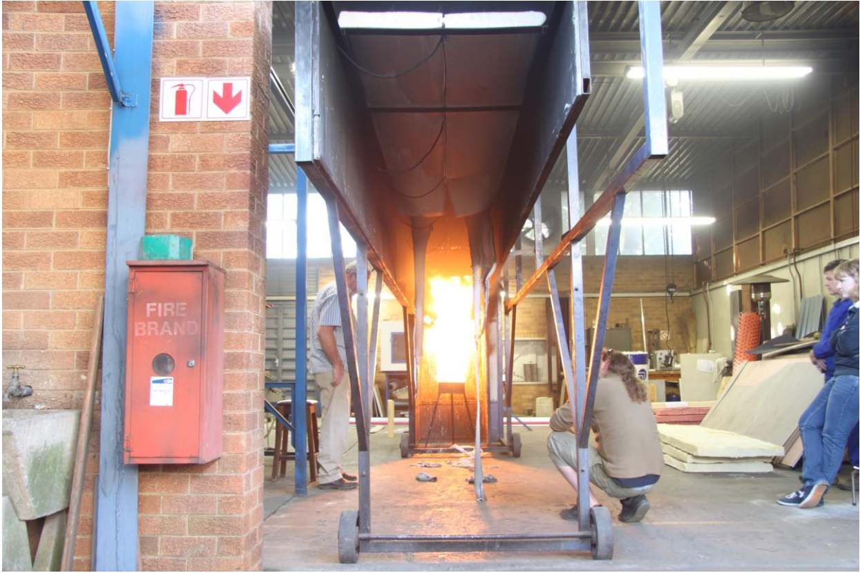
Figure 4.2.4.7: Material draping and dropping out up to 5 meter mark
