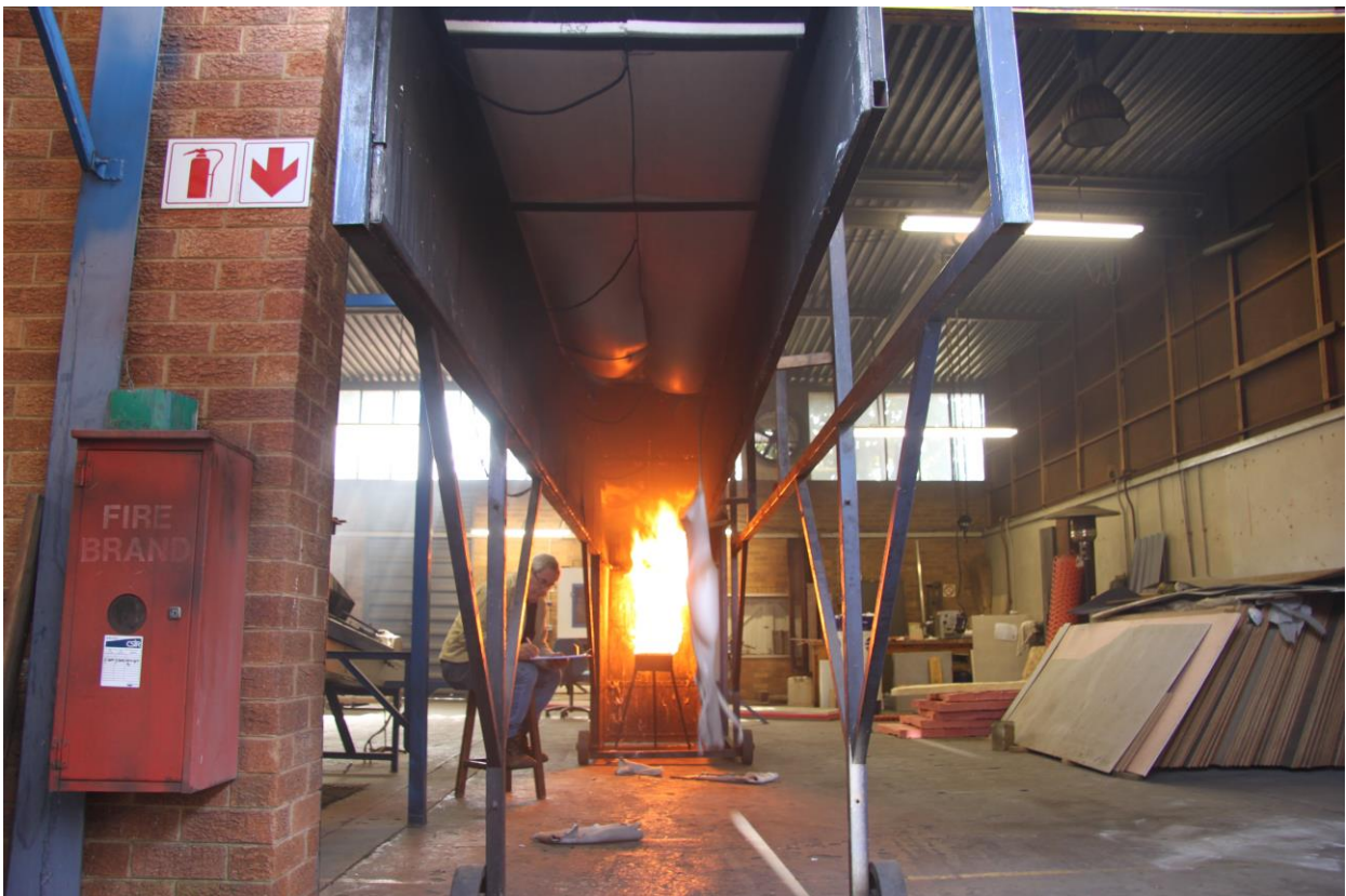
Figure 4.2.1.6: Heat damage up to 6 meter mark and dropping out up to 4 meters
