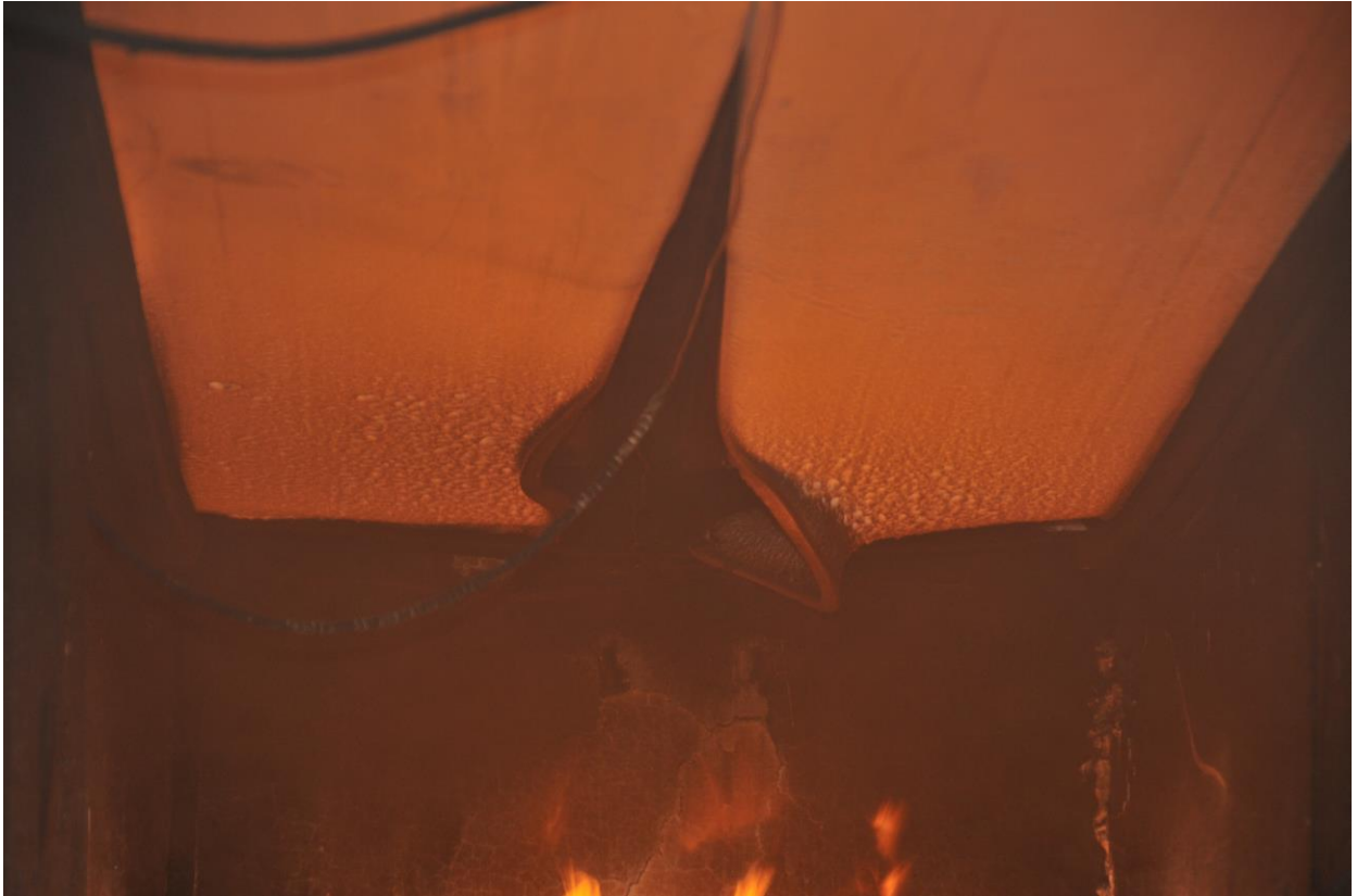
Figure 4.2.5.3: Molten material at joint starts to drape
