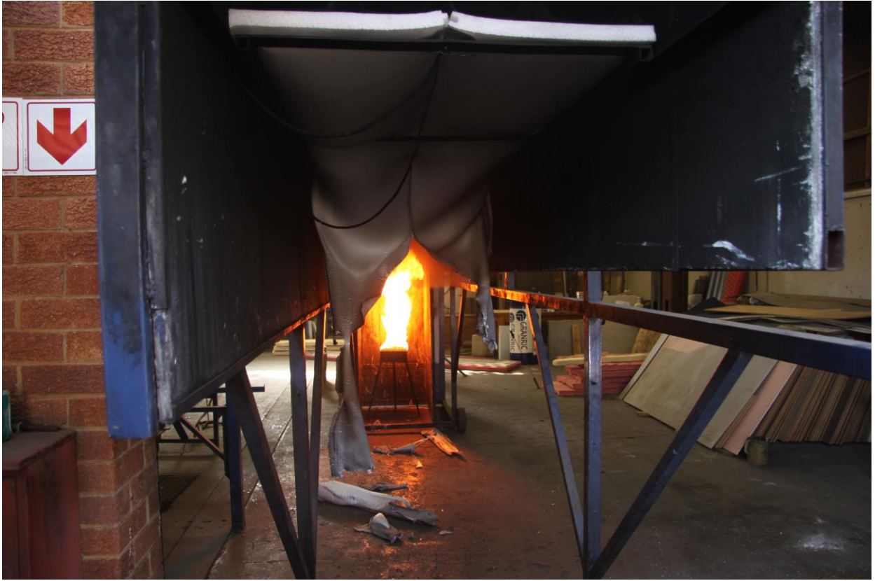
Figure 4.2.1.5: Full length heat damage with material draping out up to 6 meters
