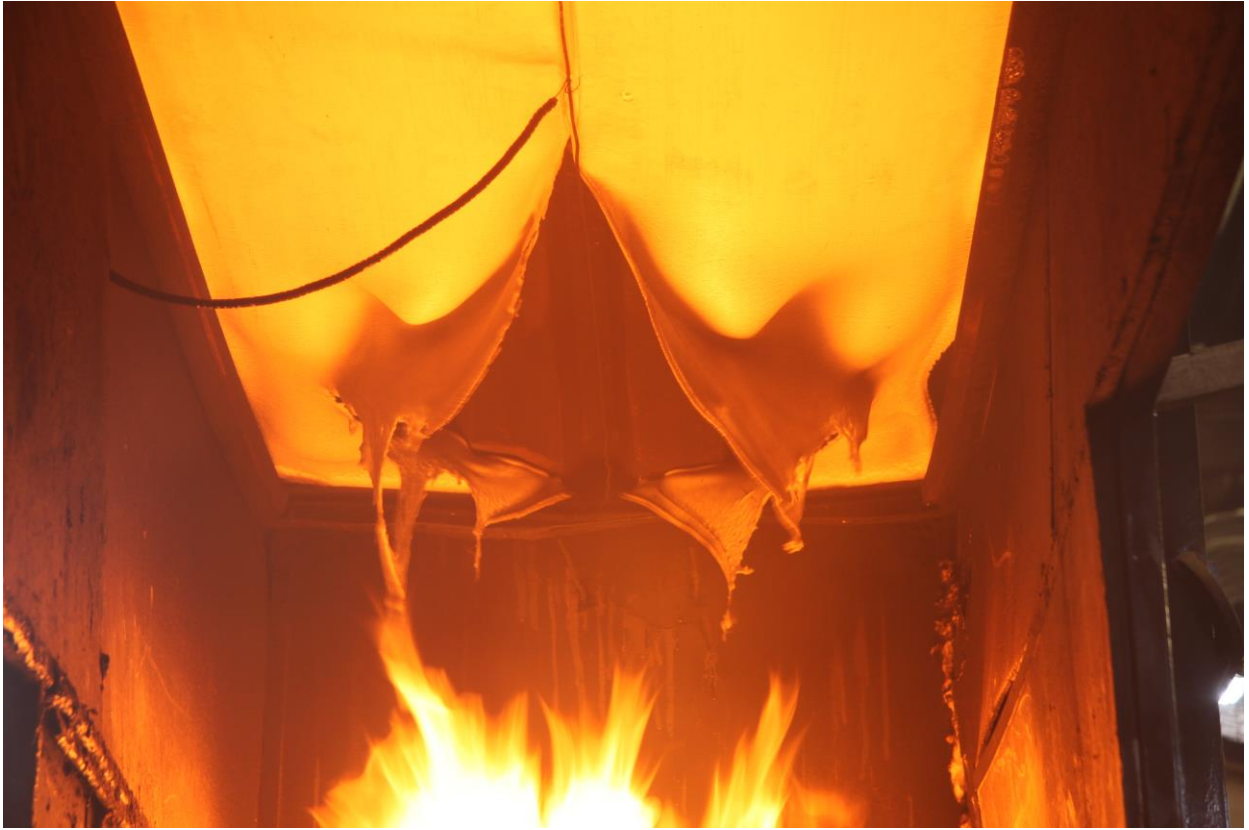
Figure 4.2.1.3: Material softening and starting to drape and drop out above the Fire Source
