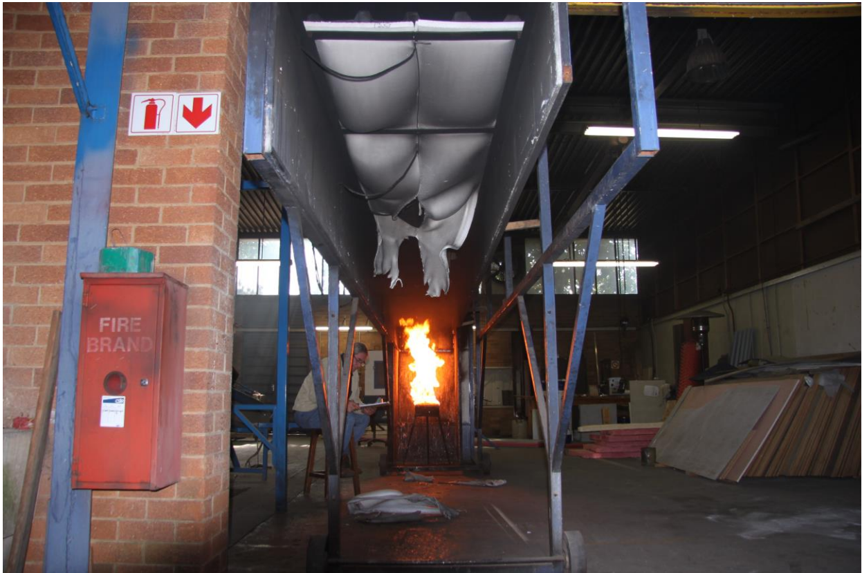
Figure 4.2.1.7: Full length heat damage with material dropping out to 4 meters
