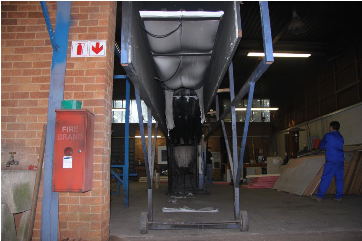
Figure 4.2.3.8: Test specimen at conclusion of SANS 10177 – 10 test
