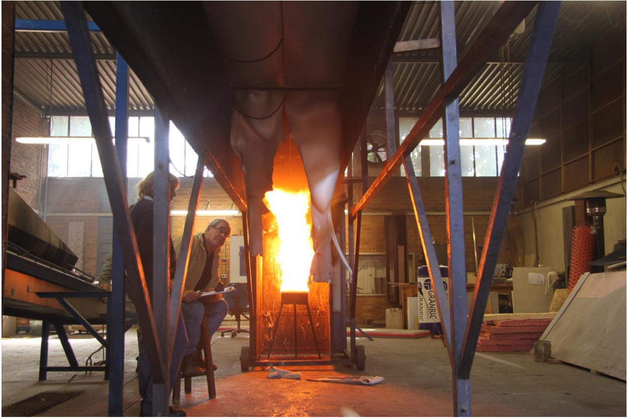
Figure 4.2.1.5: Material dropping out to 2 meter mark and draping up to 4 meters
