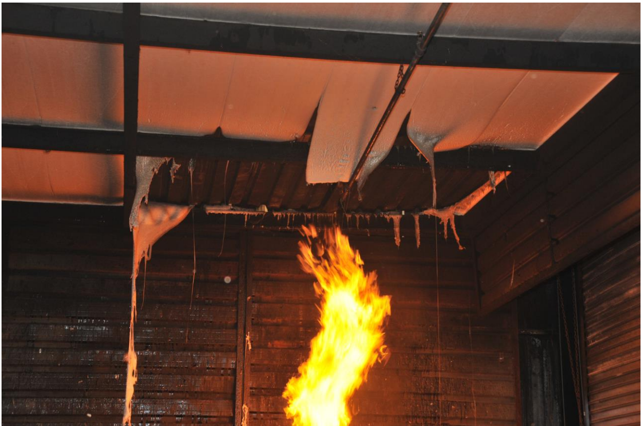
Figure 4.3.6: Boards in 2 nd bay (2 to 4 meters) starts to drape
