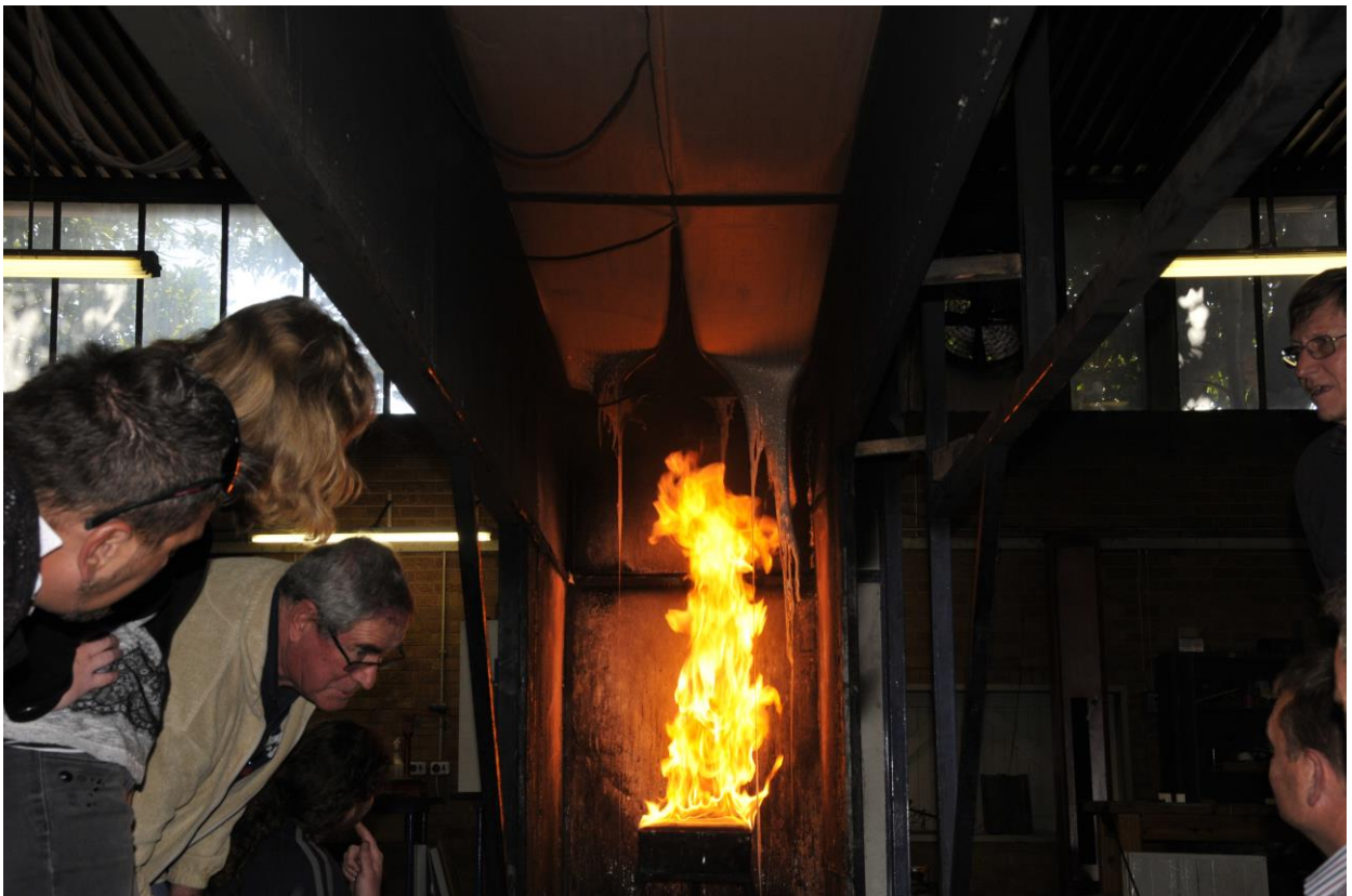
Figure 4.2.5.4: Molten material flowing out above Fire Source – Joint separated up to 2 meter mark
