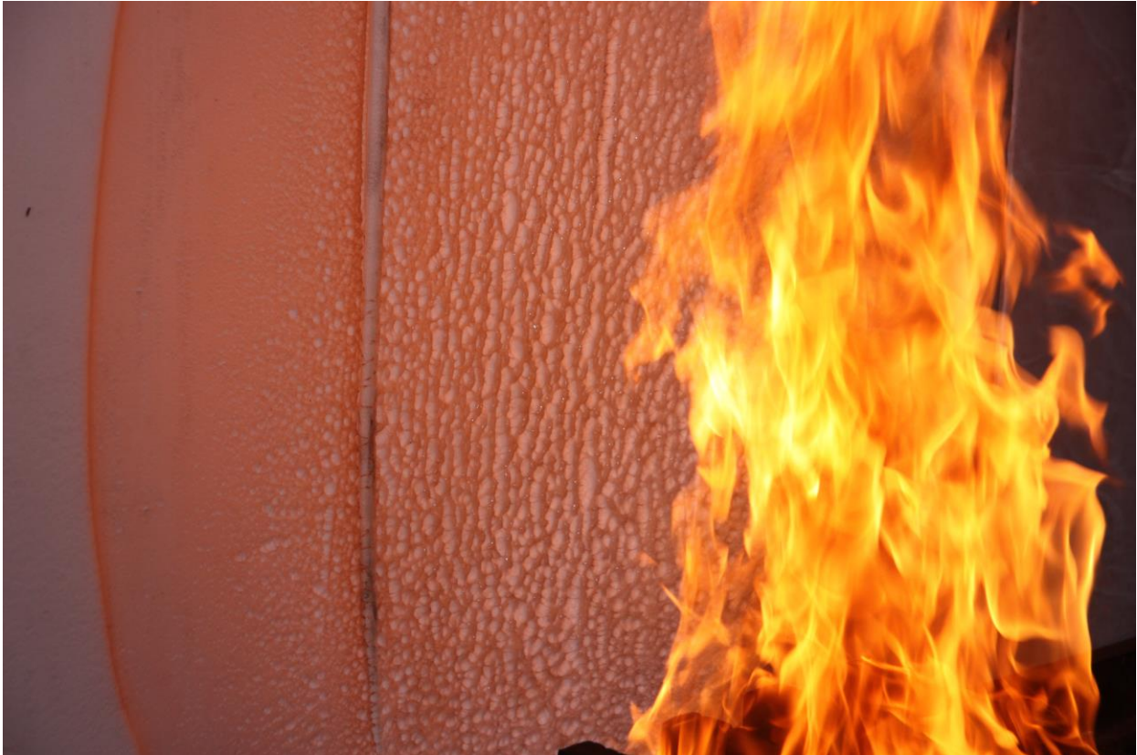
Figure 4.4.3: Coagulation of material behind Cribs
