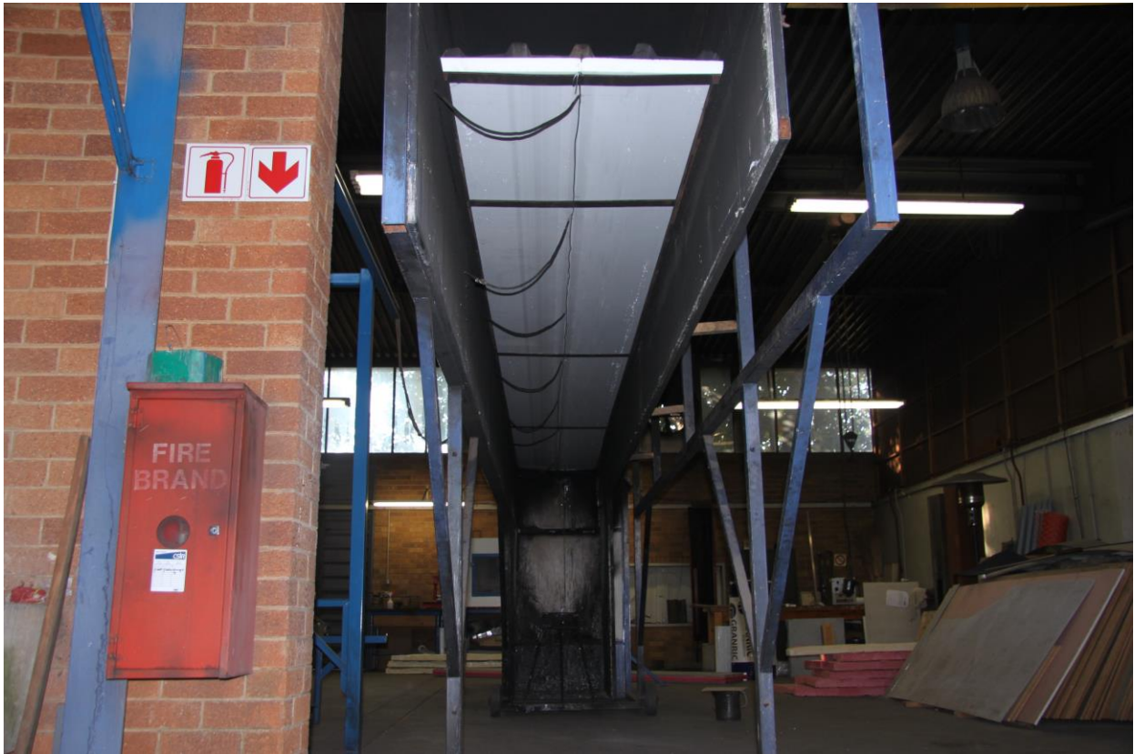
Figure 4.2.3.1: The test installation prior to ignition of the Fire Source
