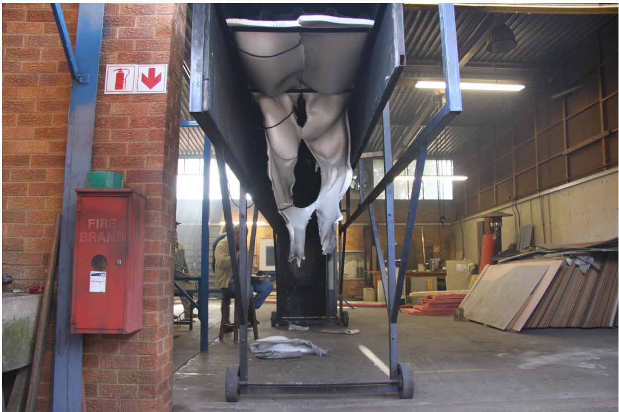
Figure 4.2.1.8: Test specimen at conclusion of SANS 10177 - 10 test
