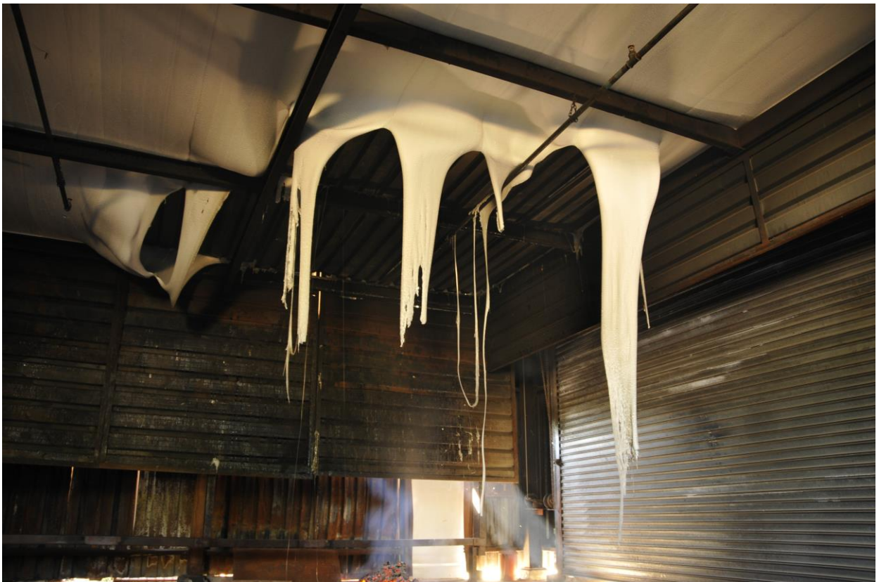
Figure 4.3.10: Test installation at conclusion of SANS 10177 – Part 11 (Horizontal) test
