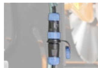
quick coupling of water pump
