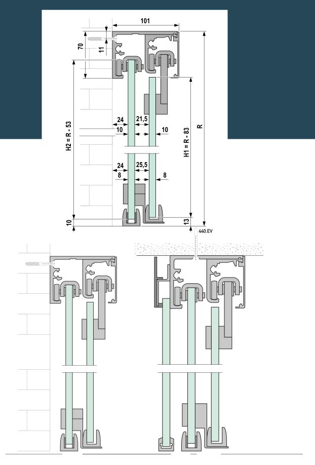
Track fixed to wall or to ceiling, fixed to ceiling with sidelight
