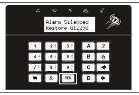
When the time is displayed, enter the number given to you by the ARC. 'Engineer Restore Performed' will be displayed.
