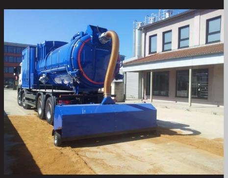
Many large industrial plants which handle bulk material, such as cement plants, require vacuum trucks in order to extract large amounts of material agglomerations, e.g. from under belt conveyors or inside process buildings. Many of these plants also need to clean the pavements and drive ways of the plant. For this, they require a road sweeper.
