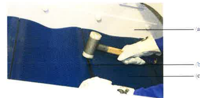
To clarify the principle, a clamped screen mat is shown here. (a) Basic construction / side wall of the screening machine (b) Clamping strip (c) Screen mat
