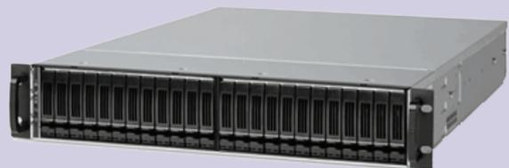
*The NX-2700 is a 2U appliance that supports 10 Mbps of WAN bandwidth and includes 1TB of secure local data store in a resilient configuration. The NX-2700 is ideal for remote and branch offices.*
