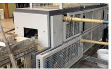
Investment has again continued at our Trafford Park Sawmills with the addition of a new mini gas dryer in December 2014. This universal vacuum coating line has an inbuilt gas infra-red dryer which enables us to dry painted materials very quickly. This means that primed and lacquered items no longer run the risk of stick marks from stacking as the items are now completely dry when they are stacked.
