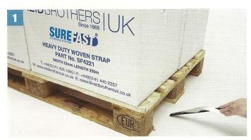
The strap must go under the pallet first by using the Surefast Pallet Lacer
