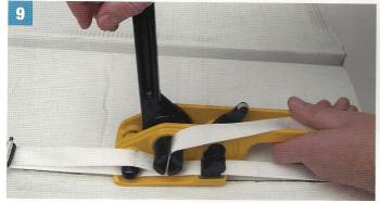
Tension the strap by rocking the handle back and froth
