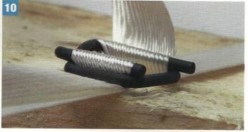
As tensioning begins, ensure that the lugs close firmly down on the strap
