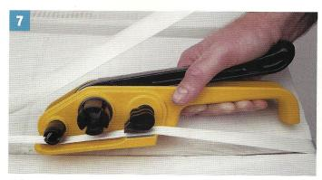
Squeeze the handle of the tensioner and place the tensioner on the bottom strap, whereby the bottom strap is set under the knife assembly and under the gripper foot
