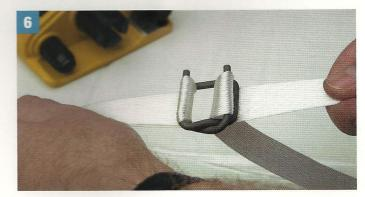
Place left hand on the bottom of the strap and pull the top strap with your right hand to make it hand tight
