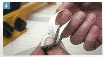
Make a new loop with the other end of the strap and lead it through the other side of the buckle, hook the loop over the other lug and pull tight
