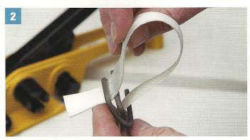
Feed the strap through the buckle as shown and pull the bottom strap with your right hand to make it hand tight leaving a 75mm tail
