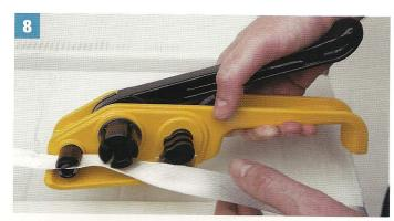
Make sure the tensioner is approximately 30cm/1 foot away from the buckle. Lead the top strap through the knife assembly
