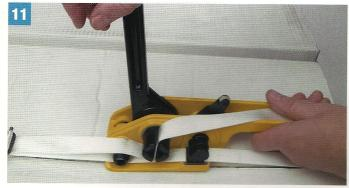
Upon completion squeeze the handle down again again to cut the strap and move tensioner away to the right
