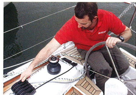
The winches look a bit small to me, but leading all the sail controls aft is a great idea
