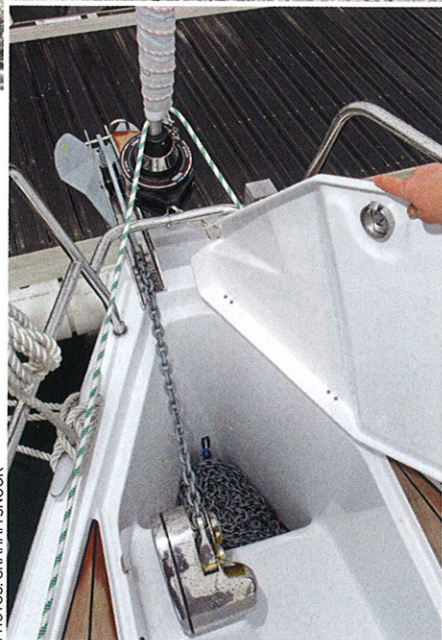
The bow roller has a padeye for a gennaker tack but no fair lead for the tack line
