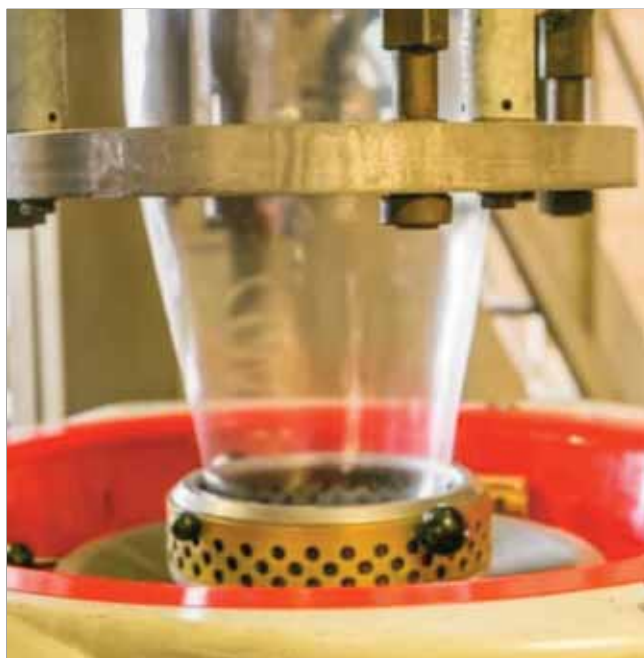
Extrusion through clear plastic film to form CO2 tubing for commercial greenhouses.
