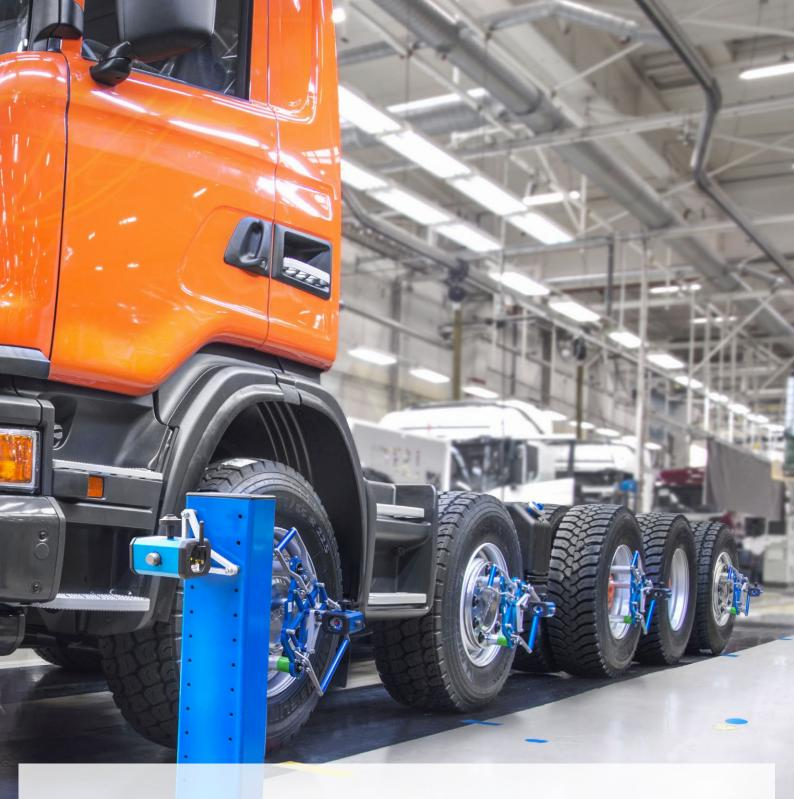
**THE ACTUAL MEASUREMENT** process starts as the operator aims the camera forward, clicks the OK-button, turns the camera to point backwards and clicks again.
