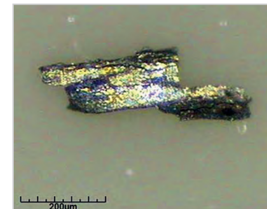
Metal particle from screw thread
