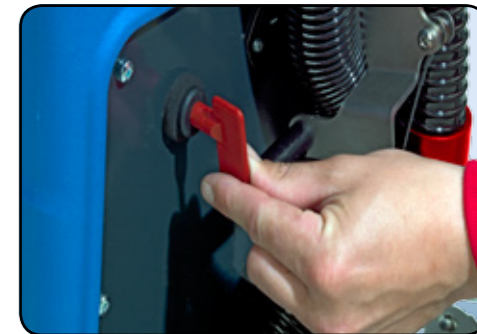
Battery isolator key
