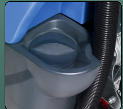
Additional fill and filter point
