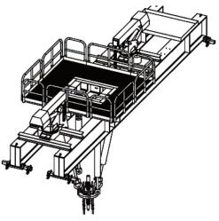
Claxton designed and built this bespoke recovery platform/false rotary at short notice to interface with the Leman platform and enable the abandonment to be carried out at a fraction of the cost of using a rig.
