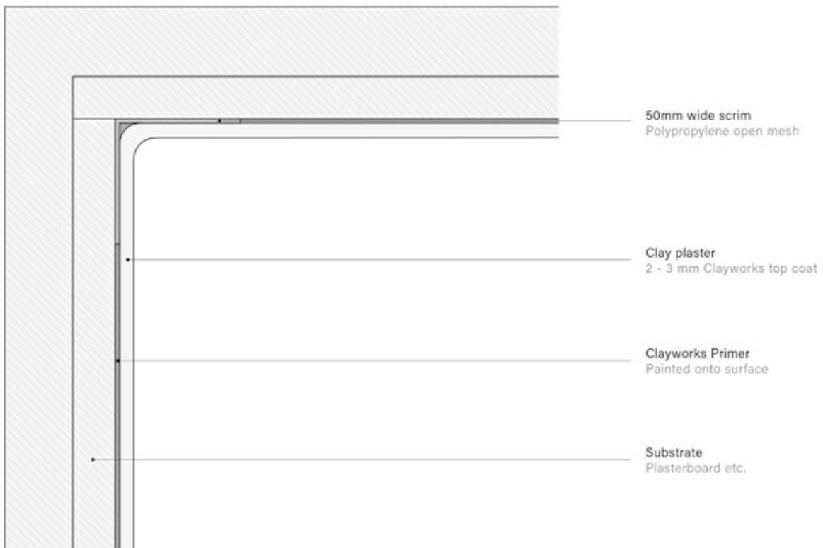
DD07 Wall-ceiling junction detail
