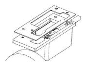
9. Observe how the shifter functions especially how the reverse selector works. The shift pattern is N-1-2-3-4-5-6.
