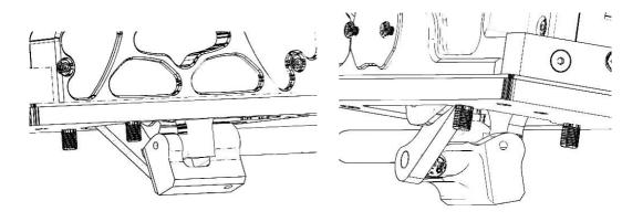
16. Fit and slightly tighten the three 8mm cap head bolts to attach the shifter to base plate then rotate the reverse selector back and forth a few times to get a feel of it.
