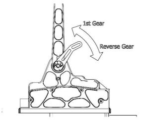
10. The reverse selection lever can be mounted facing forwards or backwards to suit the vehicle. The bolt retaining this part is held with Loctite, you will probably need heat to remove it.
