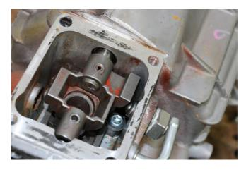
Ball plunger used to centre rod around axis, remove this and replace with bung
