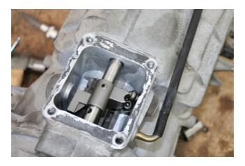
Ball plunger used to centre shaft longitudinally. Leave this in place.
