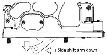
15. Slide the ball shaped fitting on the side shift arm into the groove on the left side of the shaft fitting as you lower the shifter onto the base plate. Check that the shifter slides all the way flush with the base, do not force it down with bolts
