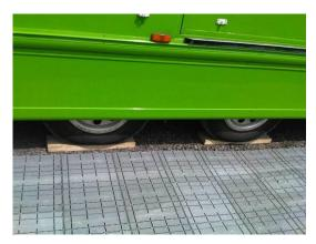
If using a floor (not supplied) this should be laid now. Ensure the floor will not restrict the securing of the awning.
