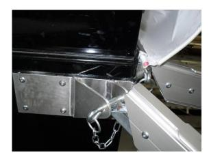
3. Starting from the main awning build the next bay along by first attaching the fascia rail (FF) to the end roof rail (SAR). Next attach the upright post (CP), ensure that one person supports this post for the next stage of the build.
