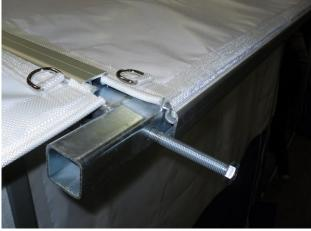
Rotate the tension beams and place over the tension brackets in the end of the roof rail. **Do not** tighten the bolts at this point. Repeat this for each bay. Tighten the bolts once all roofs are fitted.
