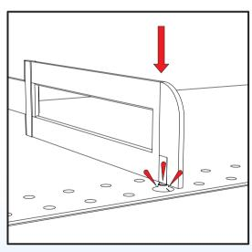
2 Insert pin into hole until it snaps in place
