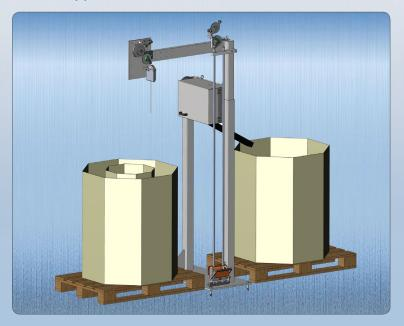
The drum with the copper wire shreds can be positioned according to layout requirements thanks to the new option.
