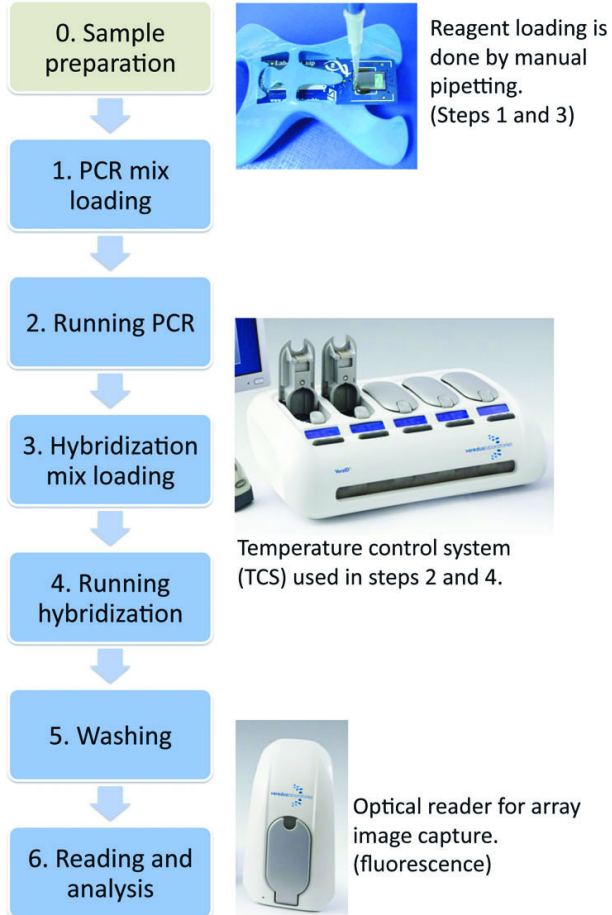
Figure 1 VereFoodborne™ assay process. 5 chips are processed in one TCS. Assay time (steps 1 to 6): 2 hrs
