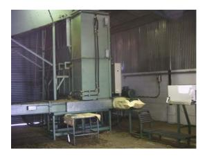
The Challenger Mass Measuring Baler has been developed to weigh, compress and bale a variety of baled materials such as chopped hay, chopped straw, shredded paper, woodchips, woodshavings, etc. They can be manufactured to a wide variety of specifications to manufacture bales with a mass of between 1 kg and 25 kg and can produce bales at a rate of up to 400 bales per hour.
