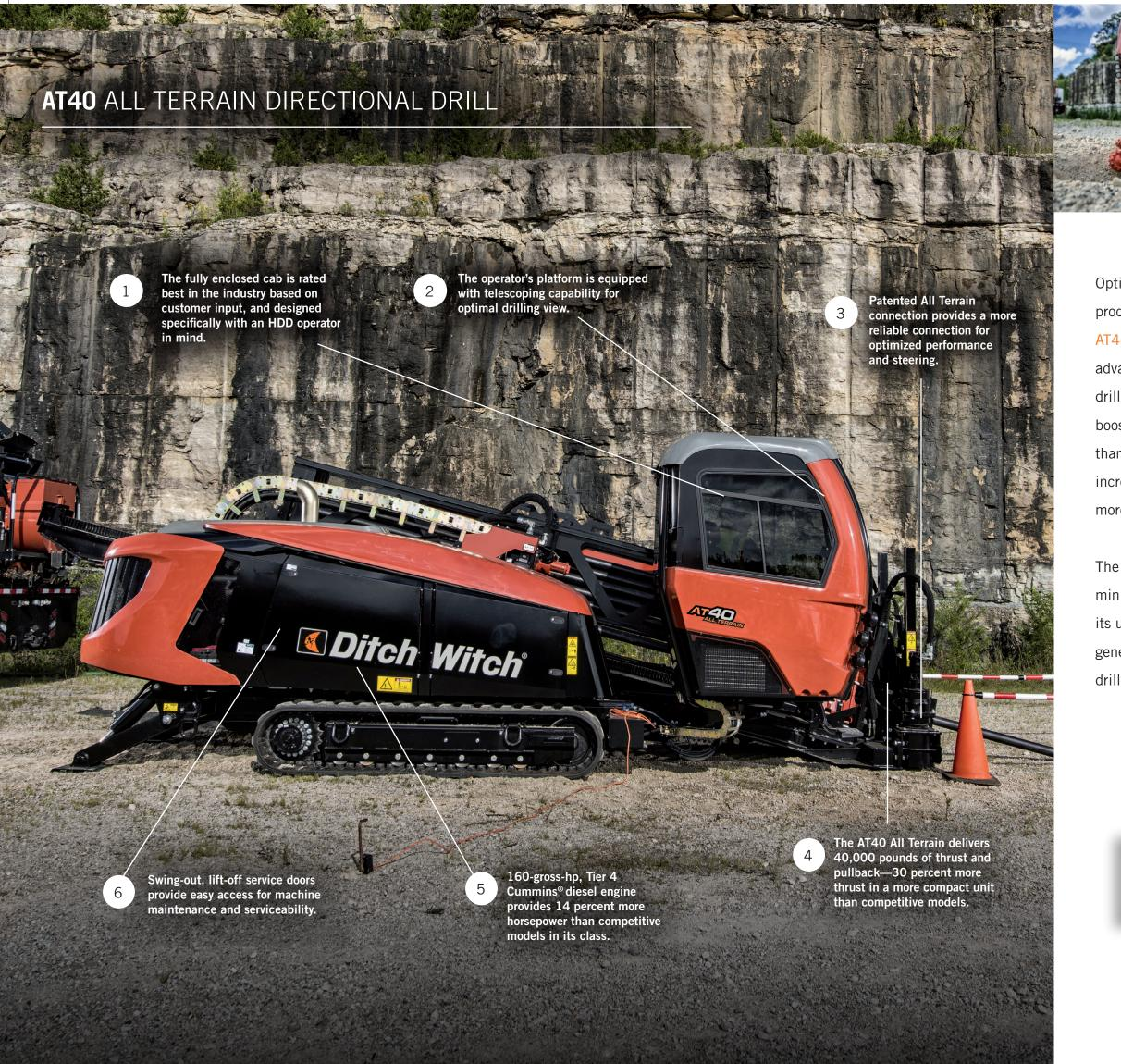
Optimized for industry-leading performance and productivity in hard rock conditions, the Ditch Witch® AT40 All Terrain directional drill is designed with an advanced version of the proven Ditch Witch All Terrain drilling system. The updated, two-pipe system offers boosted power to the bit—33 percent more torque than competitive units. Patented design enhancements increase cycle times, improve durability and allow for more adaptable steering.
