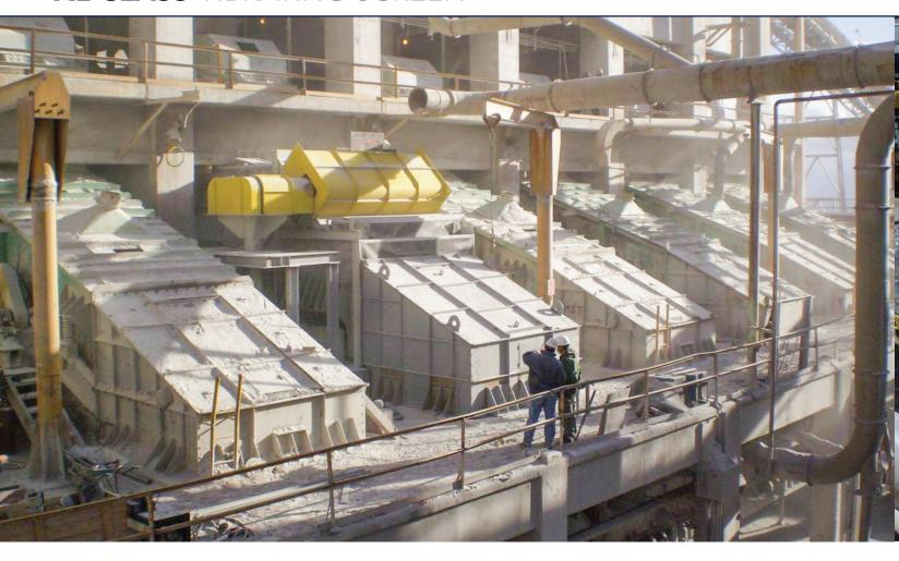
The Niagara XL-Class vibrating screen combines advanced exciter drive technology with a wide body to offer better screening action and more throughput. It is intended for high tonnage production rates, yet designed for low maintenance, easy operation and unmatched reliability.
