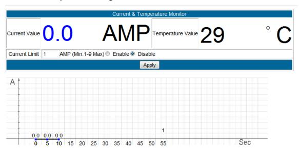
**Current Value:** Show the consume ampere of the device connected with **9255Pro**. The tolerance of the current measurement is plus or minus at 10% degree.
