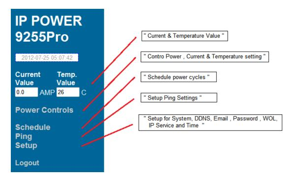
**Current & Temp. value :** show the consume current ampere and internal temperature at Celsius.
