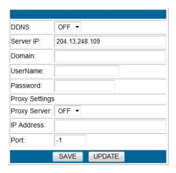
**DDNS Server IP:** The DDNS server IP **Domain:** Type in the dyndns domain name **Username:** Enter the DDNS username here **Password:** Enter the DDNS password.
