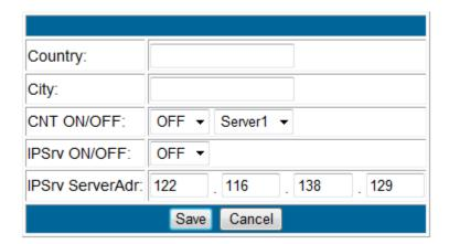
IP service allows you to easily find your device of the web or of the google cloud server without the need to remember long IP Addresses. Instead you can find your device easily just by searching with the name of your device.
