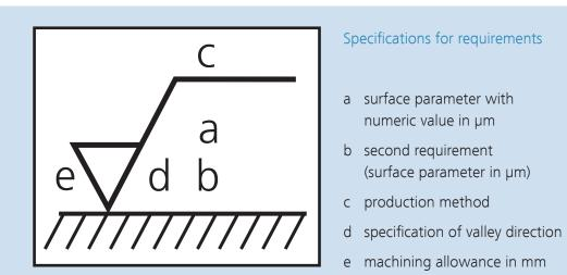
surface parameter with numeric value in µm second requirement (surface parameter in µm) production method
