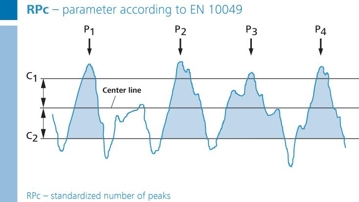
RPc corresponds to the number of local peaks, which successively exceed an upper section line c1 and a lower section line c2. The number of peaks is related to a length of 10 mm irrespective of the evaluation length selected.
