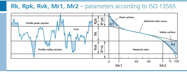
Parameters of the material ratio curve
