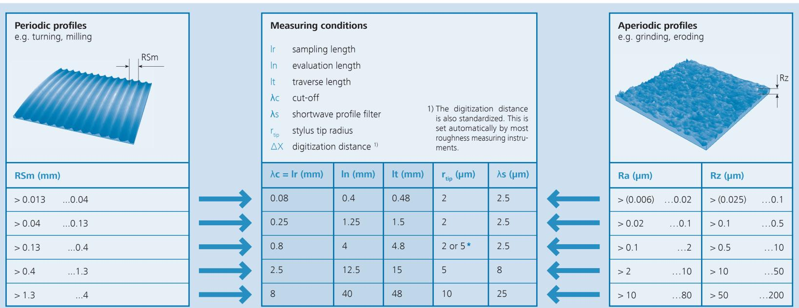
In a periodic profile the mean width of the profile elements RSm is used. With an RSm between 0.4 and 1.3 mm the following measuring conditions result:  $\lambda c = 2.5 \text{ mm} / \ln = 12.5 \text{ mm} / \ln = 15 \text{ mm} / r_{tin} = 5 \mu \text{m} / \lambda s = 8 \mu \text{m}$ .
