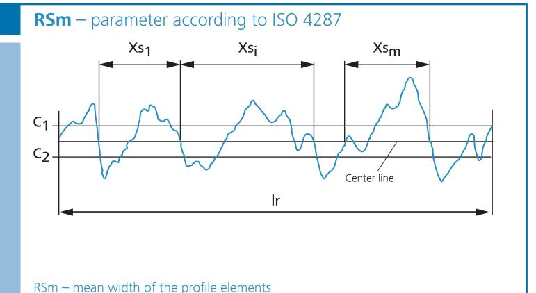
RSm is the arithmetic mean value of the width of the roughness profile elements within the sampling length and requires the definition of height discriminations (c1, c2) matching the function of the surface.
