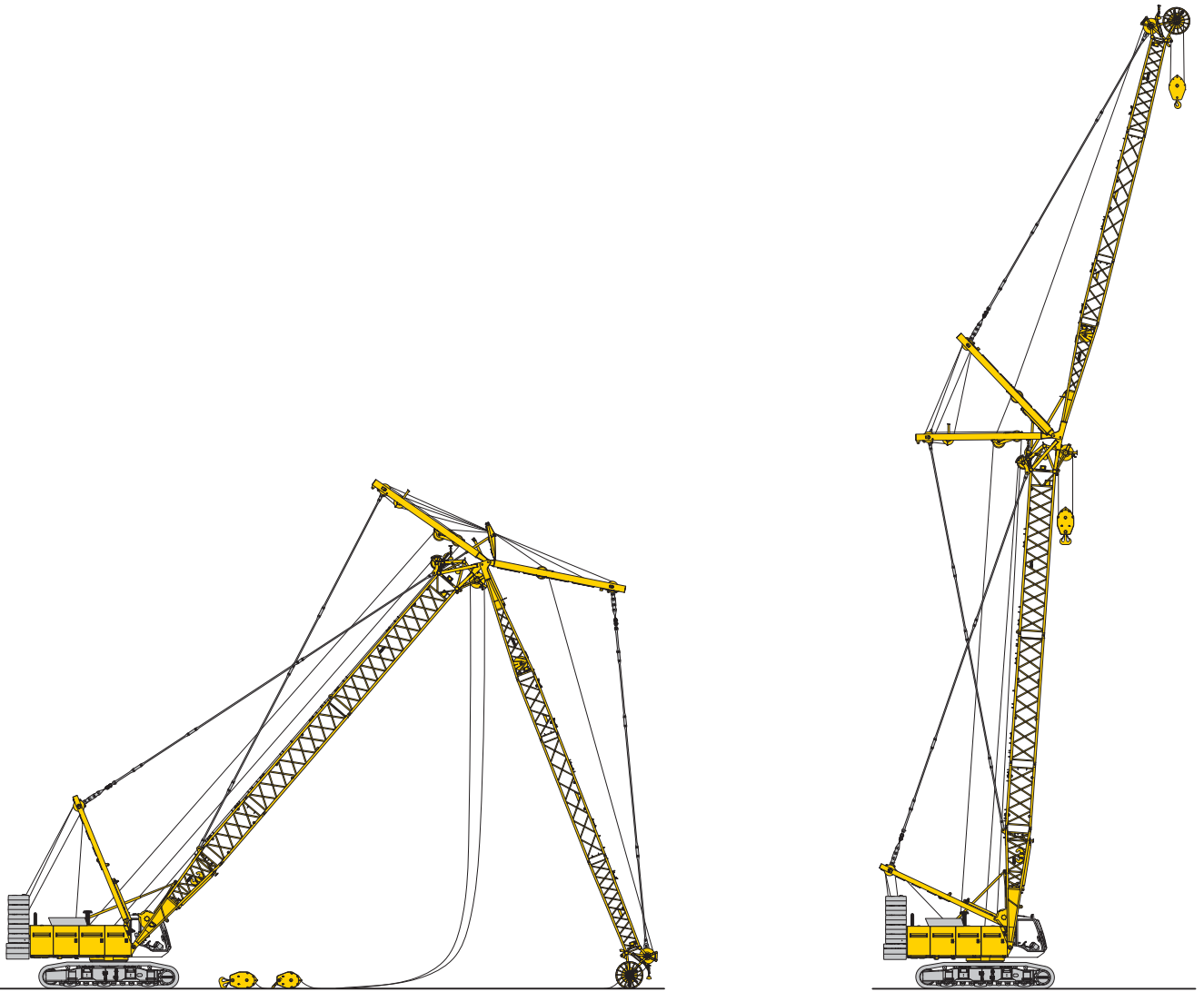
Erecting of main boom and luffing jib
