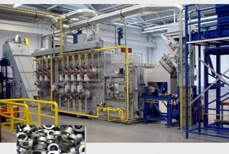
for hardening and tempering of hot forged parts
