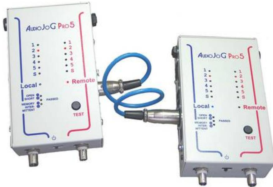
1. Set up the Remote end first by pressing and holding the Test button whilst switching the tester on. Plug the cable under test in the appropriate socket on the 'Remote' side of the unit.
