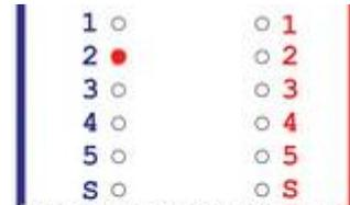
Fig 9. OPEN circuit at Pin 2 (Local)
