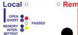
c) A short to SCREEN, this may be indicated by one, or both the screen LED's being ON in conjunction with another pair of LED's (Fig10).
