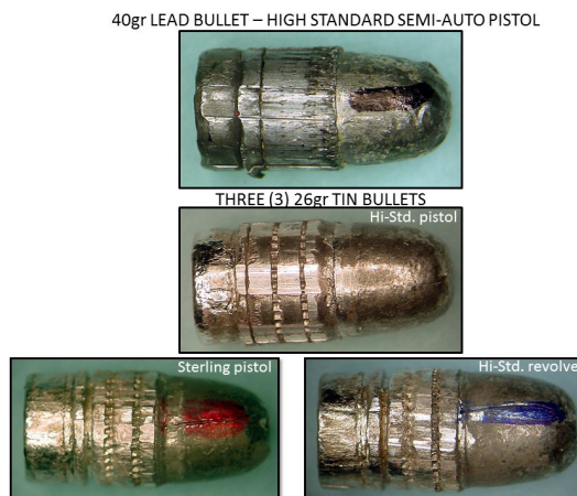
Figure 8: Lead bullet from High Standard pistol (top) and tin bullets from three handguns
