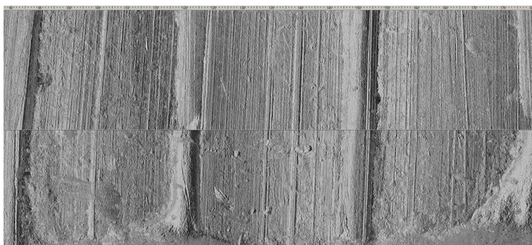
Figure 9b: High Standard Sportking pistol best match on a land impression – 150% image – lead bullets
