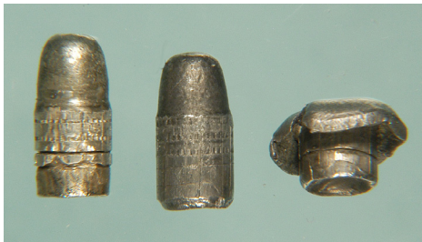
Figure 5: Bullets recovered from a block of Clearballistics Upper – Win. X22LRHLF 26-gr Tin HP Middle – Win. Wildcat 40-gr LRN Lower – Win. Xpert22 40-gr LHP
