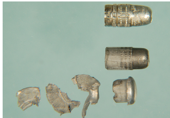
Figure 4: Bullets recovered from a block of ballistic soap Upper – Win. X22LRHLF 26-gr Tin HP Middle – Win. Wildcat 40-gr LRN Lower – Win. Xpert22 40-gr LHP
