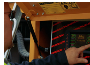
User friendly waterproof and dustproof control panel. Allows monitoring of pressures, fluid levels and fuel consumption. Provides push button control of jaw, track and feeder functions.
