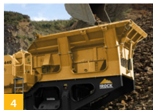
4 Folding HARDOX® hopper mounted over vibrating pan feeder built with steeper angles to reduce material sticking. Feeder rate regulated manually or automatically by load sensing jaw.
