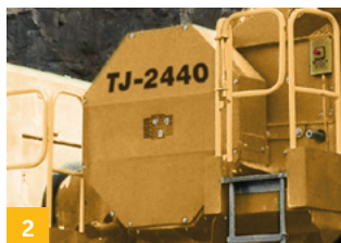
2 True 40" x 24" jaw with reversible hydrostatic drive, reversible jaw plates, and fully hydraulic closed side setting (CSS) adjust.
