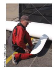
Above The Infusion's 'gybing' daggerboards have a thicker trailing edge at the top, allowing them to twist in their cases and provide extra lift upwind.
