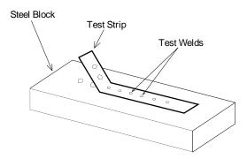
Figure 3 - Peel Test
