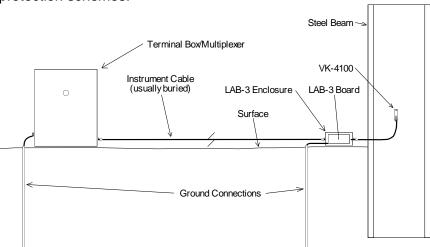
Figure 11 - Lightning Protection Scheme
