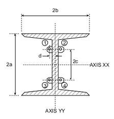
Figure 13A - Strain Gages Mounted on Central Web Axial Strain and Bending Moments about both XX and YY Axes (Recommended)
