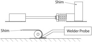
Figure 7 Welding the Collar Shim in Place.
