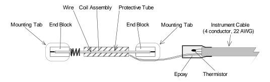
Figure 2 - VK-4150 Vibrating Wire Strain Gage
