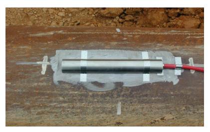
Figure 9 - Spot welded cover plate
