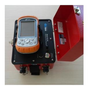
Figure 12 GK405 Readout Unit
