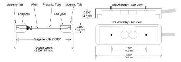
Figure 1 - VK-4100 Vibrating Wire Strain Gage and Coil Assembly
